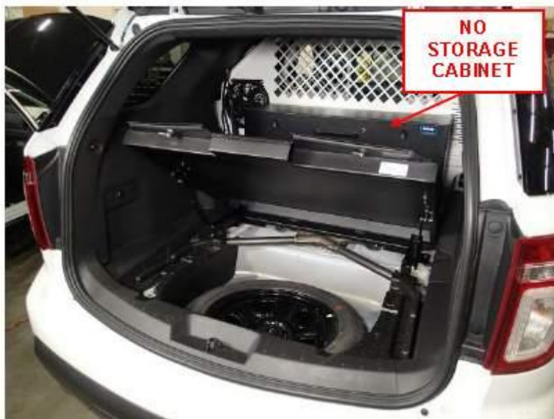
Figure 28B – Havis Products – Installation de plaque de chargement articulée
