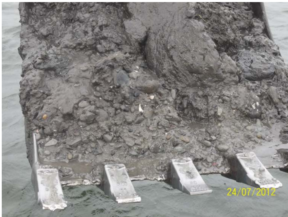
Photo 7 - Dark silt with some organics some gravel encountered at TP 3 - McEachern's Point (Elevation -1.00 to -1.80 CD).
