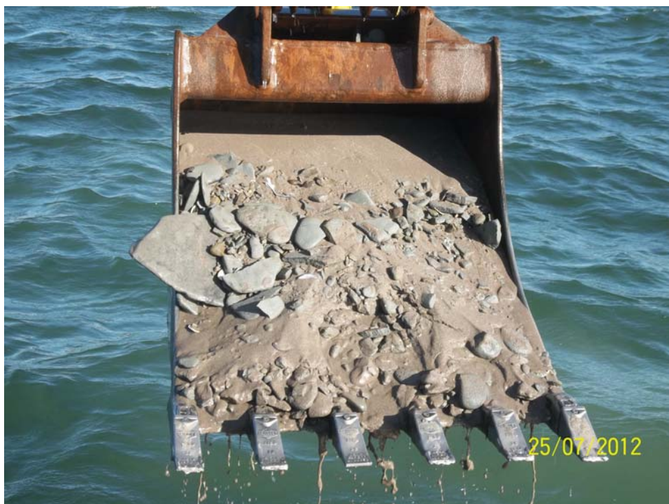
Photo 18 - Brown sand and gravel with some cobbles and flat boulders encountered at TP 14 - McEachern's Point (Elevation -0.90 to -2.60 CD).
