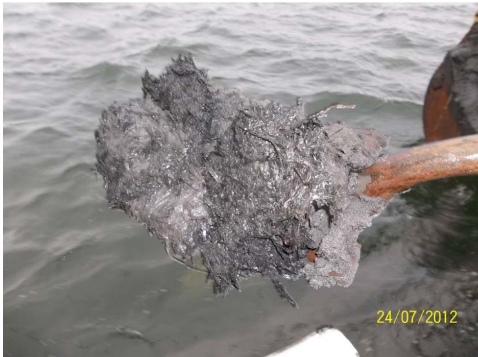
Photo 8 - Organics present in silt layer at TP 4 - McEachern's Point (Elevation -1.21 to -2.21 CD).
