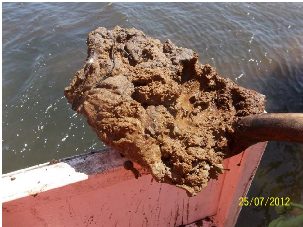
Photo 12 - Orange brown sand with some gravel encountered at TP 8 – McEachern's Point (Elevation -1.35 to -1.85 CD).
