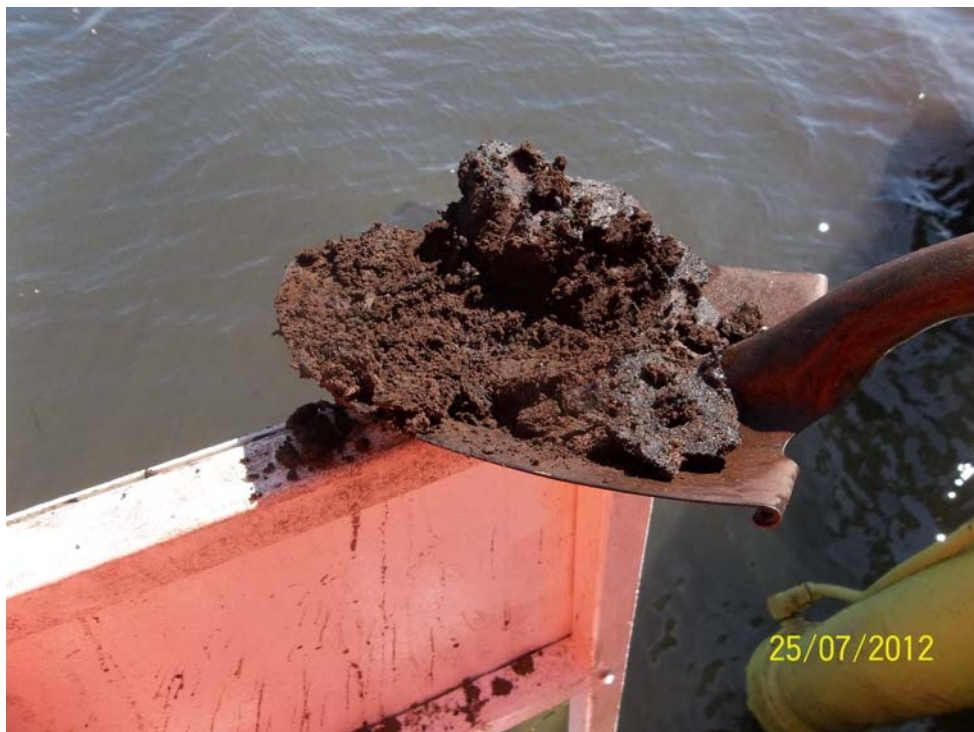
Photo 13 - Peat encountered at TP 9 - McEachern's Point (Elevation –1.58 to –1.73 CD).
