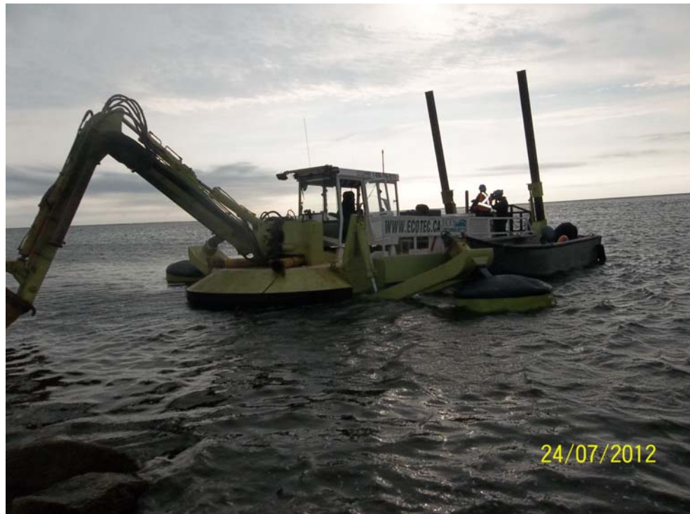
Photo 2 - Amphibian excavator in McEachern's point channel.
