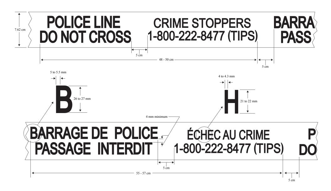
Unless otherwise indicated, all measurements are subject to  $\pm$  1.0 cm tolerances. Tape width tolerance to be  $\pm$ 2 mm.
