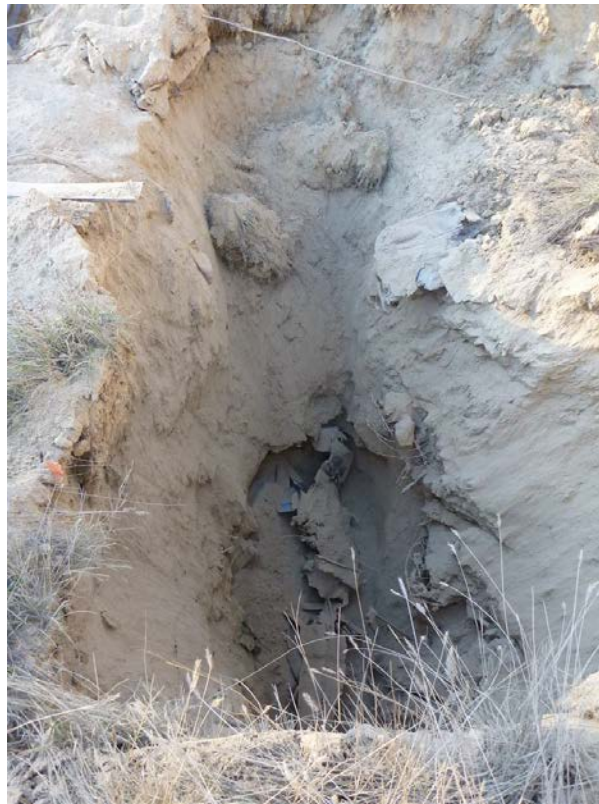
Photo 21: TP8 – Debris encountered to 4 m.
