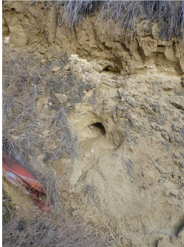
Photo 57: Void outlet and saturated soil (March 2014)
