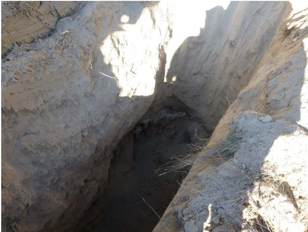
Photo 8: TP2 – At 4 m metal debris still encountered.
