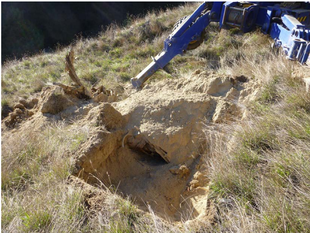
Photo 20: TP8 – Debris observed at 0.5 m.
