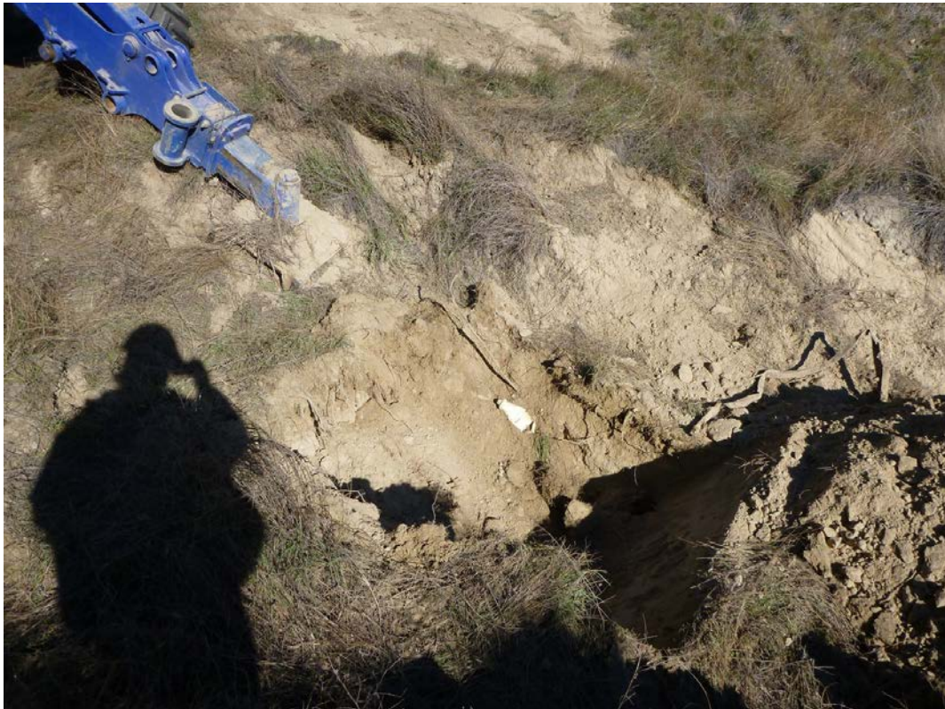
Photo 14: TP7 – debris observed at 0.5 m.
