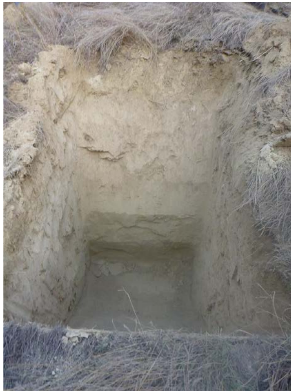
Photo 28: TP10 – Excavated test pit up to 3 m.
