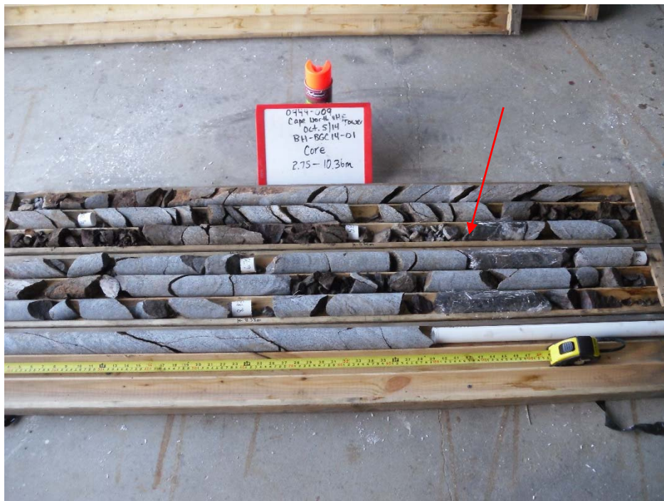
Photo 6: Shows the core retrieved in the borehole from approx. 2.8 m to 10.4 m depth. The borehole depth of 5.9 m is indicated by the Red Arrow on Photo.
