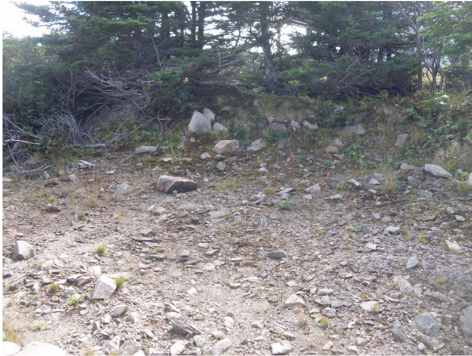
Photo 3: Shows earth-cut, with angular gravel, cobble and boulder particles at surface.
