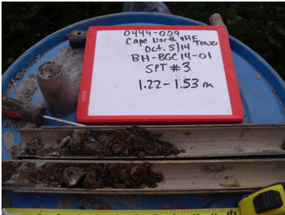
Photo 2: Shows the Glacial Till sampled from depth of 1.22 – 1.53 m below ground surface. Poor recovery apparent in split spoon apparatus.
