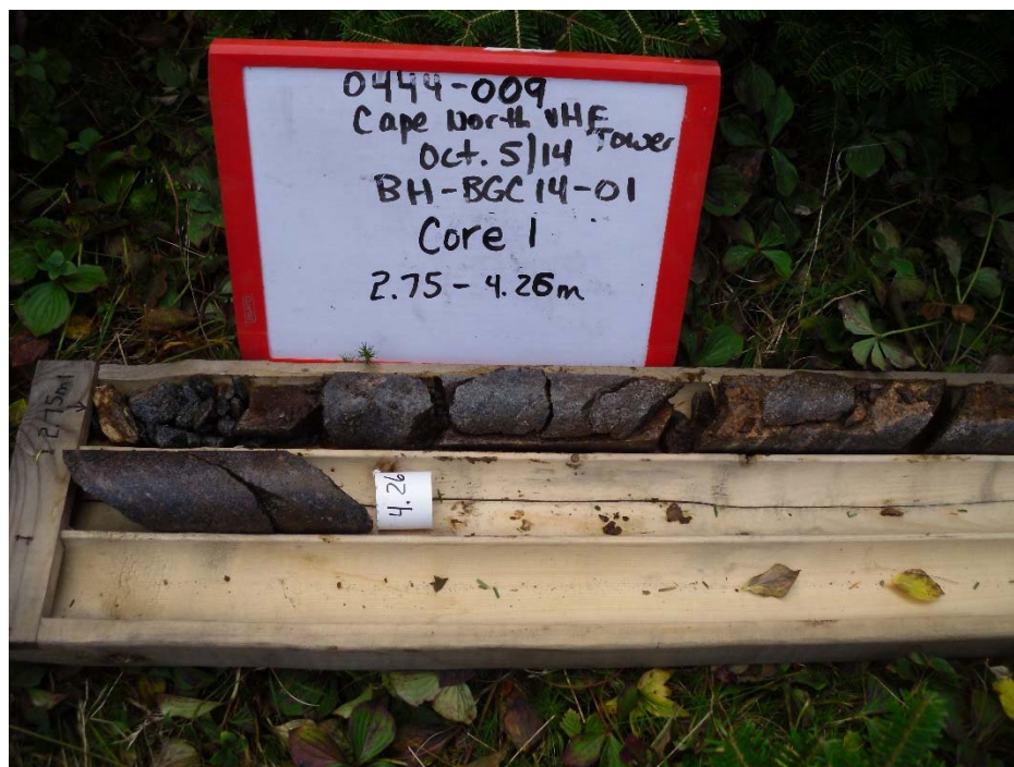
Photo 4: Shows zone of weathered bedrock.
