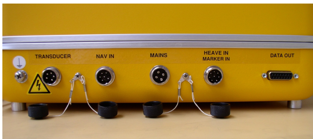
Figure 1-3 Output connectors
