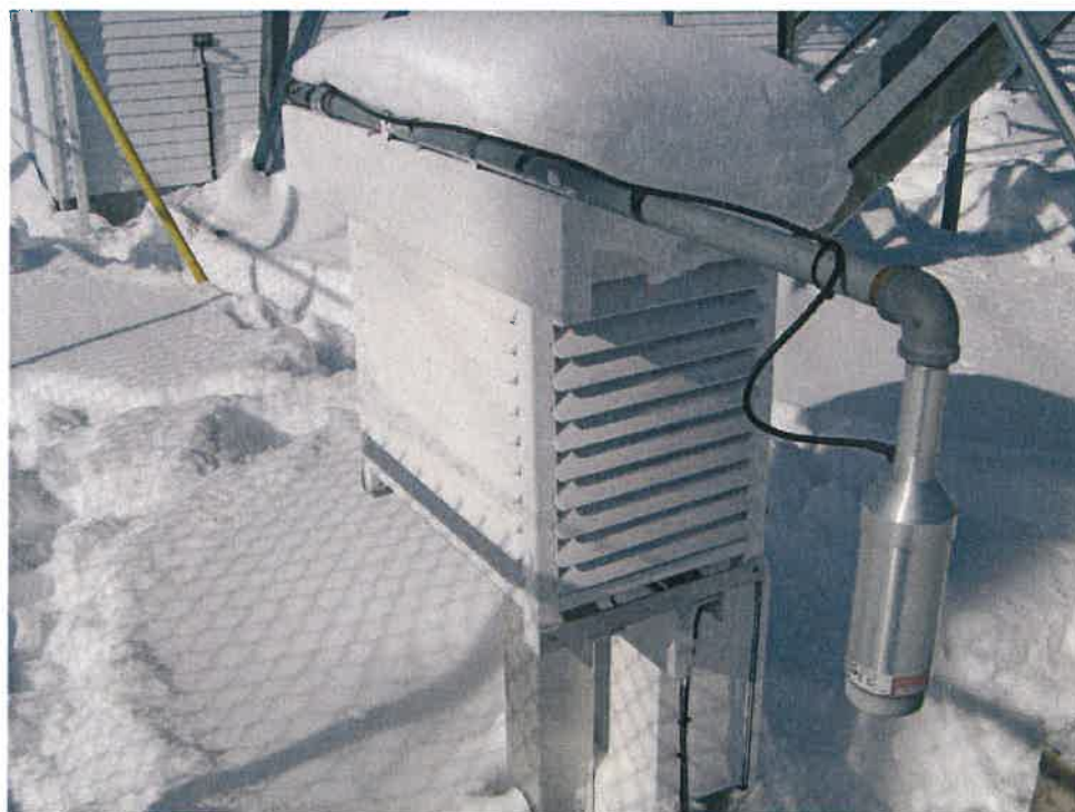
Photo #16: Un-Protected Snow Meter
