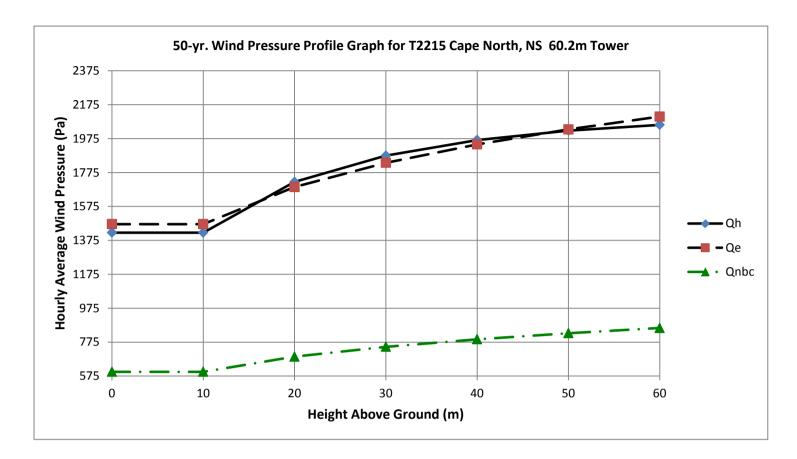
Qe profile = Qe (the site-specific equivalent reference wind pressure) with the 2/10 power law profile.
