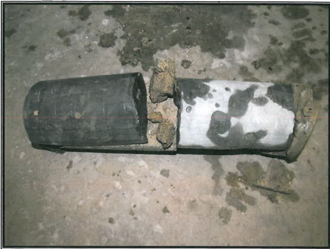
Picture 7 : Sample from the right wall from the exterior stone facing of the east building. (2013-06-06)
