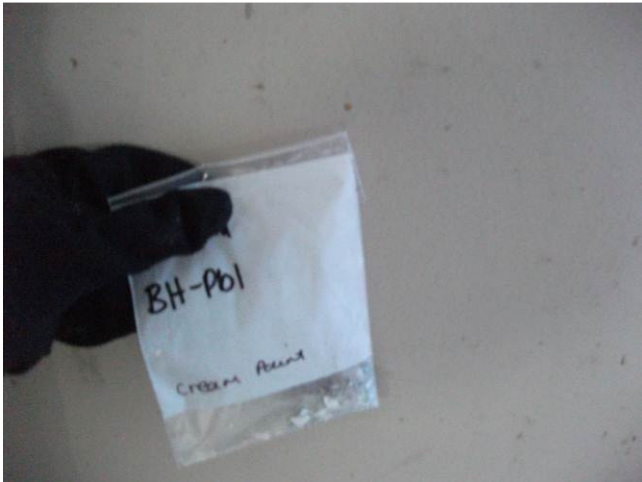
Photograph 27: Boat House Building – Lead-Based Cream Wall Paint
