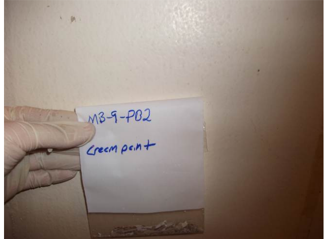
Photograph 2: Main Building- PB2 – Lead-Based Cream Paint Undercoat Throughout Main Building
