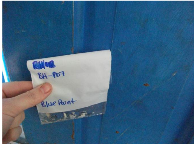
Photograph 30: Boat House Building – Lead-Based Blue Wall Paint
