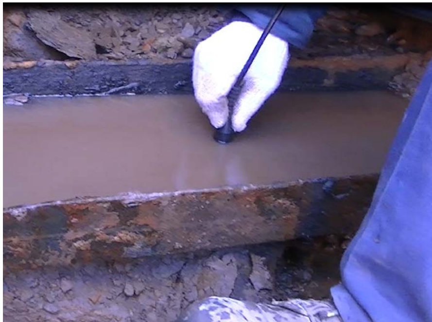
Photo 56 – Ultrasonic thickness testing.
