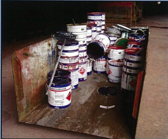
Residual paint in the cans, may drip out of the skip and enter the marine environment through the drain systems.
