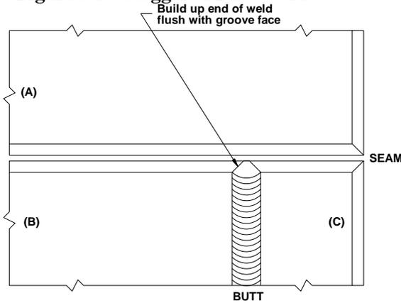
**Figure 5.6 Aligned Butt Weld**
