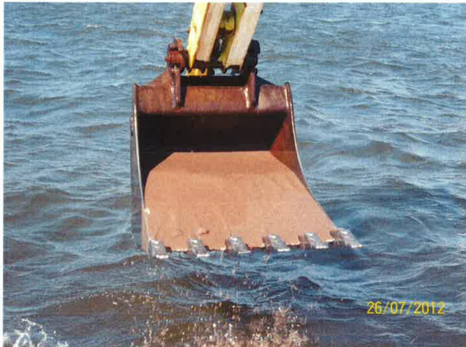
Photo 14 - Brown sand with some gravel and occasional cobbles at TP 10 - Pigeon Hill (Elevation - 0.93 to -3.13 CD).
