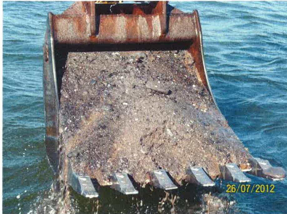
Photo 15 - Grey sand and gravel with some cobbles and occasional boulder at TP 11 - Pigeon Hill (Elevation -0.70 to -2.80 CD).
