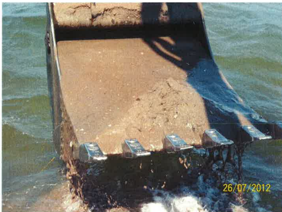
Photo 6 - Brown sand with trace silt, gravel and organics at TP 2 - Pigeon Hill (Elevation -0.64 to -2.94 CD).
