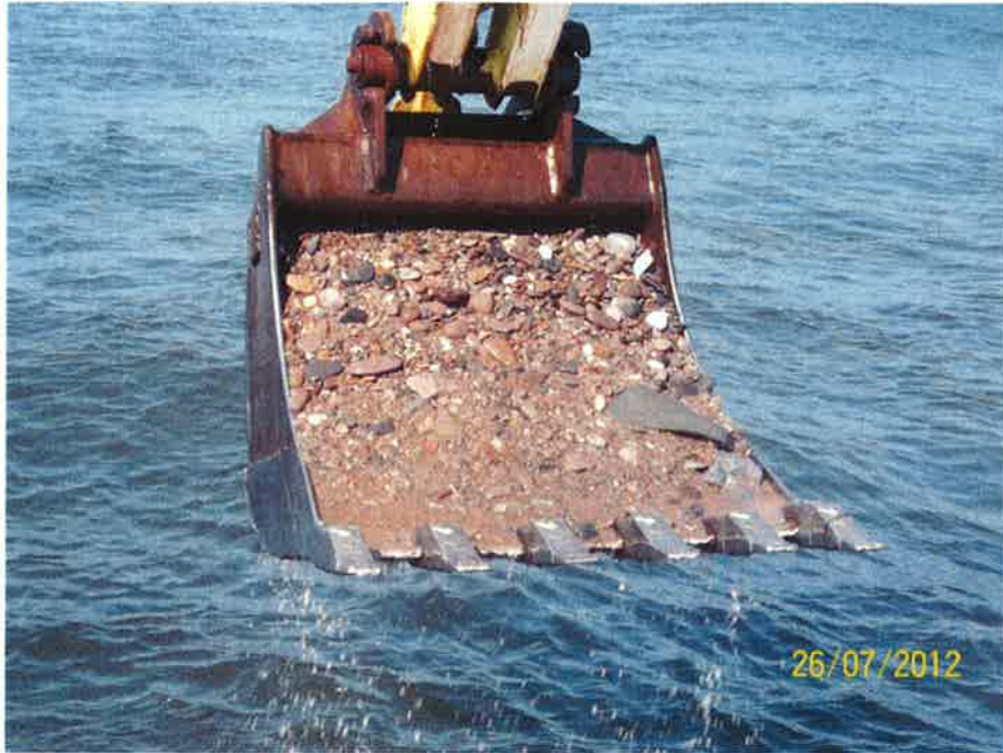
Photo 13 - Gravel with some sand and some cobbles and boulders at TP 9 - Pigeon Hill (Elevation - 0.79 to -2.69 CD).
