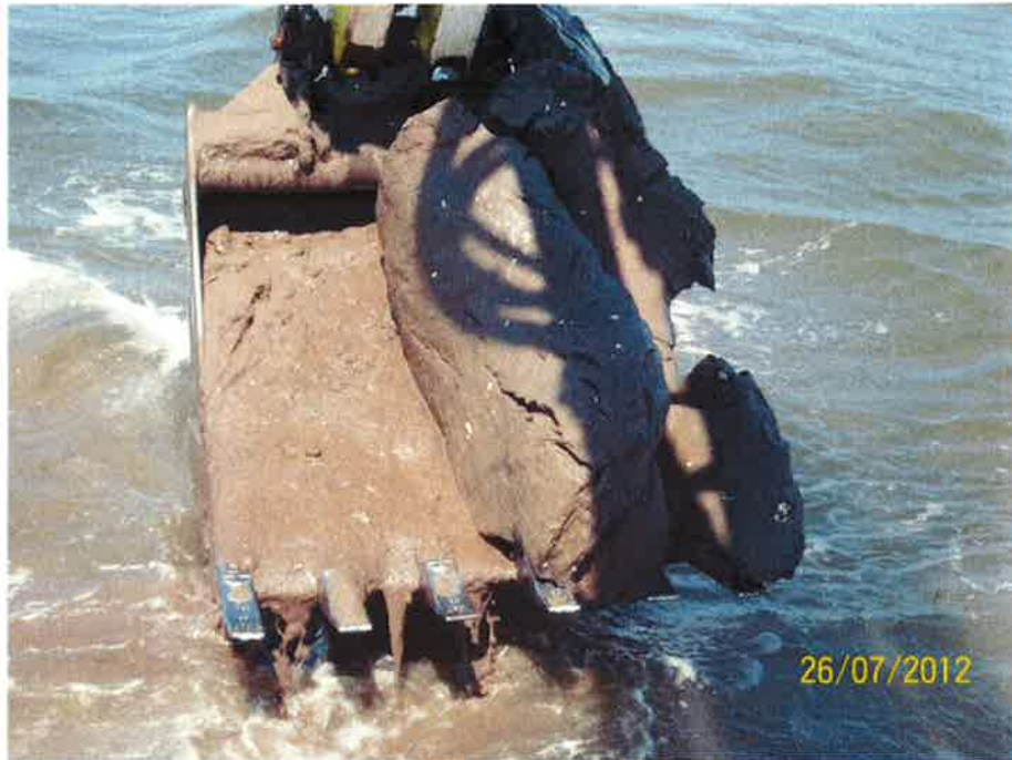
Photo 7 - Brown sand with trace silt, gravel, and organics at TP3 - Pigeon Hill (Elevation 0.08 to -1.32 metres CD).
