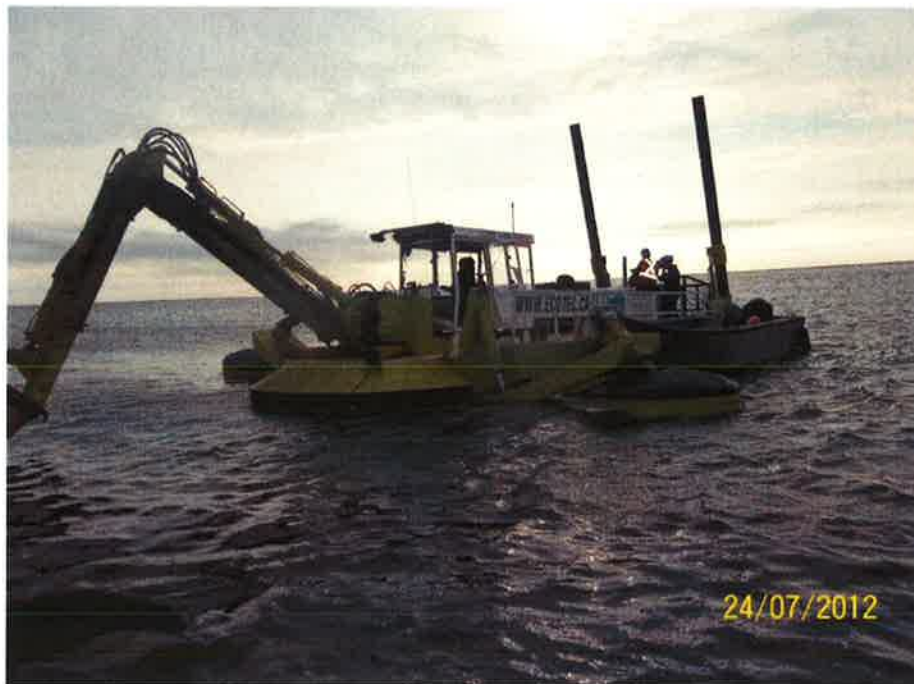
Photo 2 - Amphibian excavator in McEachern's point channel.
