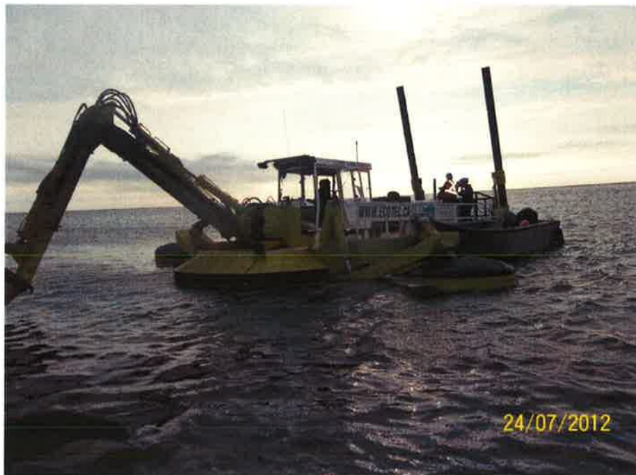
Photo 2 - Amphibian excavator in McEachern's point channel.
