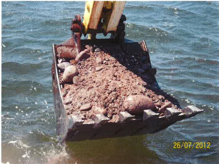
Photo 9 - Brown gravel with some snad, cobbles and boulders at TP 5 - Pigeon Hill (Elevation -1.13 to -2.63 CD).
