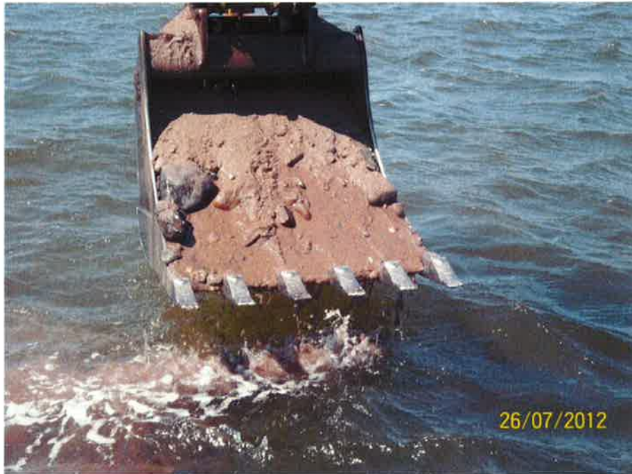
Photo 11 – Brown sand and gravel with cobbles and boulders at TP7 - Pigeon Hill (Elevation -0.94 to -2.74 CD).
