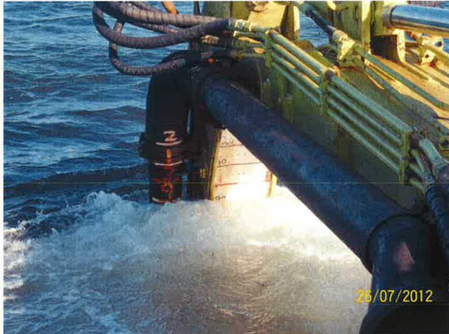
Photo 4 - Depth during excavation tracked by sounding measurements on inside of excavator arm.
