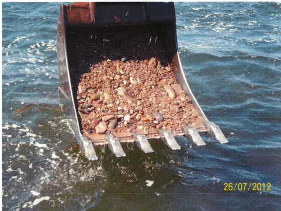
Photo 12 - Gravel with cobbles and some sand and occasional boulder at TP 8 - Pigeon Hill (Elevation -0.83 to -1.53 CD).
