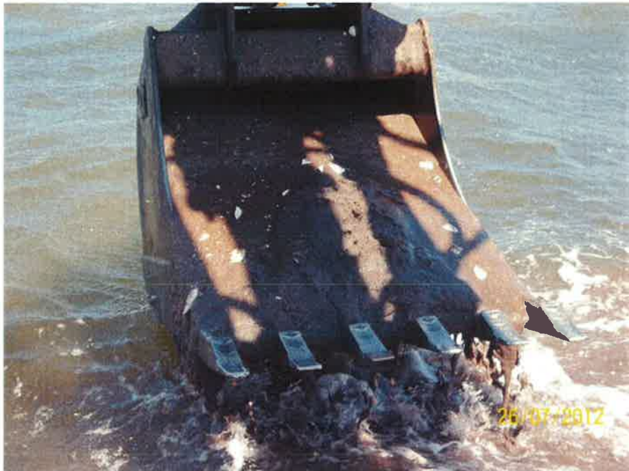
Photo 8 - Sand with some gravel and trace silt and organics at TP 4 - Pigeon Hill (Elevation -1.15 to -2.75 CD).
