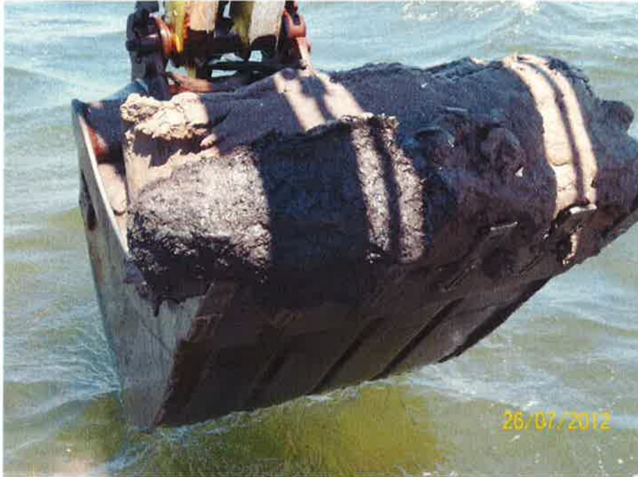
Photo 5 - Dark grey silty sand with organics at TP 1 - Pigeon Hill (Elevation -1.31 to -1.61 CD).
