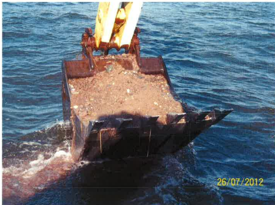
Photo 16 - Sand and gravel with some cobbles and occasional boulders at TP 12 - Pigeon Hill (Elevation -0.57 to -2.77 CD).
