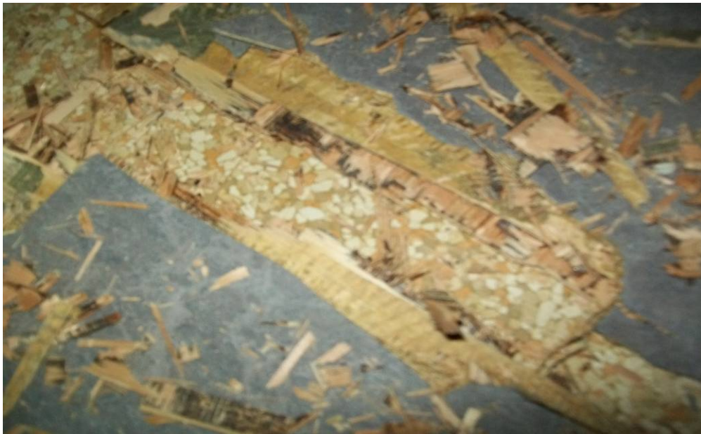
Photograph 4: View of asbestos-containing vinyl sheet flooring (VSF4) (white speckled) along floor of east wing of building. Sample (VSF4-01a) contained 20% Chrysotile asbestos.
