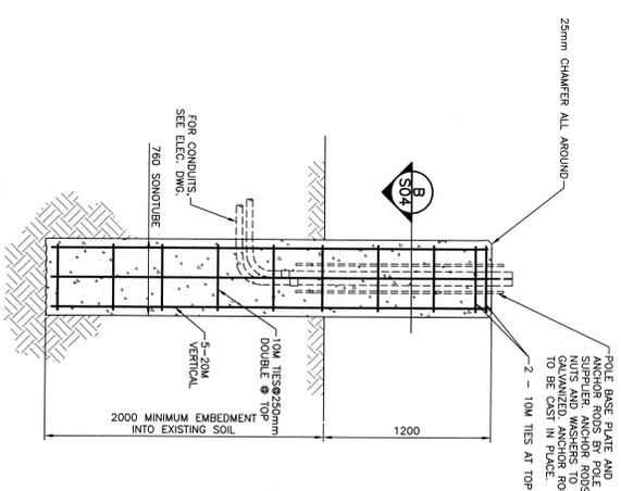
TYPICAL POLE MOUNTED LUMINAIRE BASE
