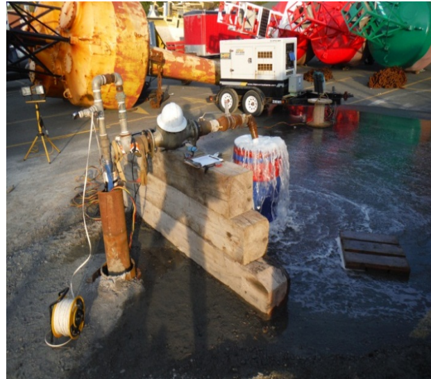
Photo 2 Aquifer testing setup at Well 1
