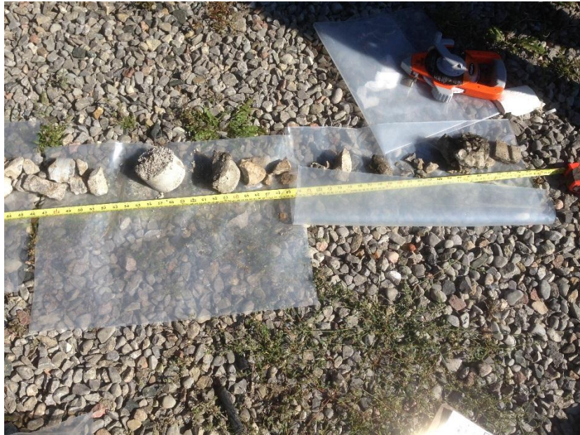
Photograph 7: Corehole CH 13-3 Rock Fills or Highly Weathered Rock Pieces
