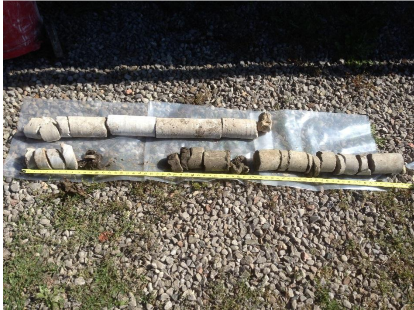
Photograph 3: Corehole CH 13-2 Concrete Cores and full depth Rock Cores
