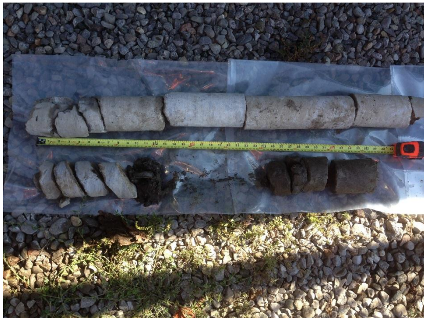
Photograph 4: Corehole CH 13-2 Concrete Cores and zone of clayey silt within the limestone rock
