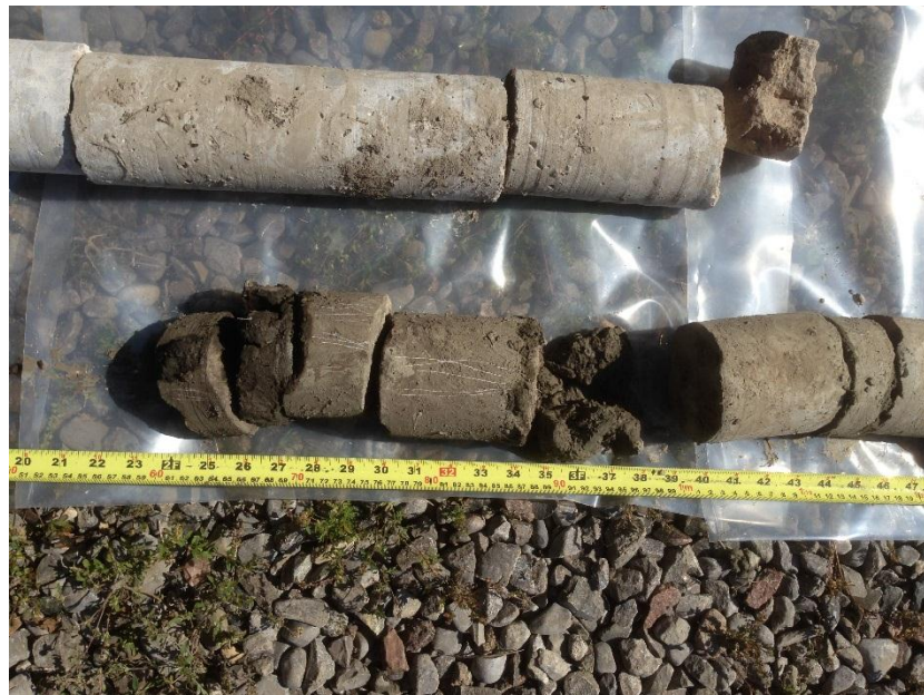
Photograph 5: Corehole CH 13-2 Layers of clayey silt within the limestone rock
