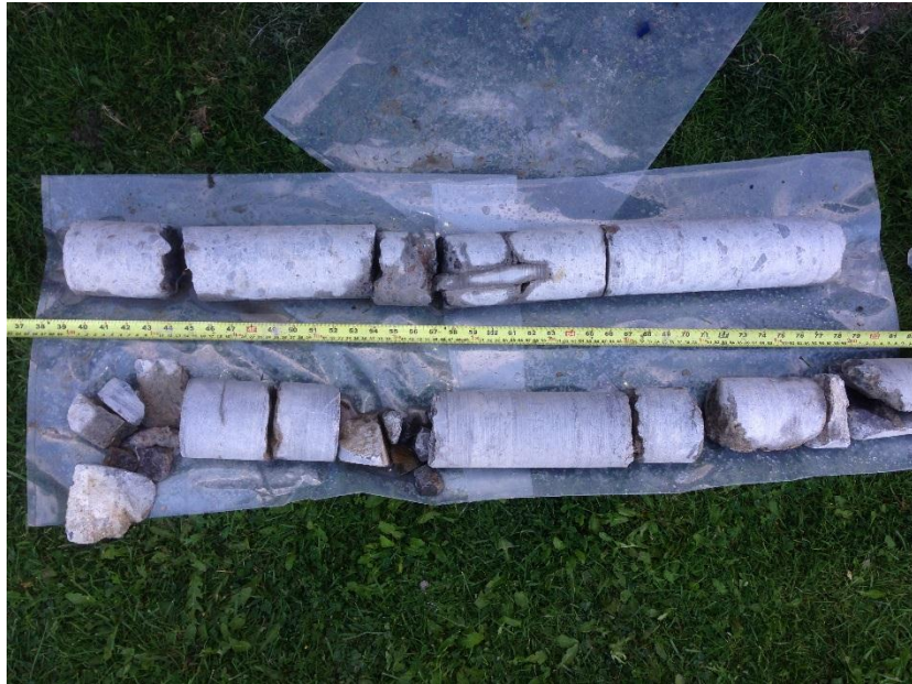
Photograph 1: Corehole CH 13-1 Concrete Cores and partial Rock Cores
