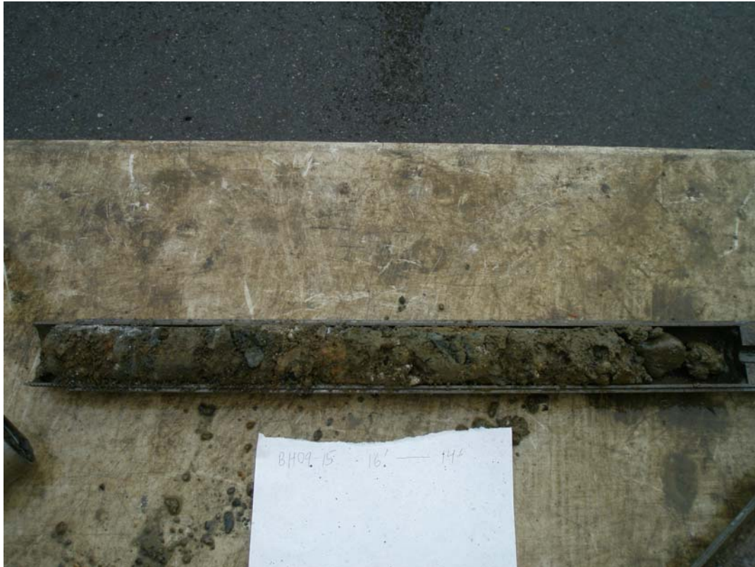
Photograph 15: Borehole soils encountered in BH09-15 from 4.3 m to 4.9 m depth.
