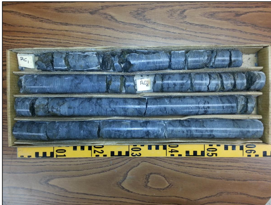
Photo 9 - Grey limestone bedrock cored between 0.9 to 3.1 m depth at BH 7.
