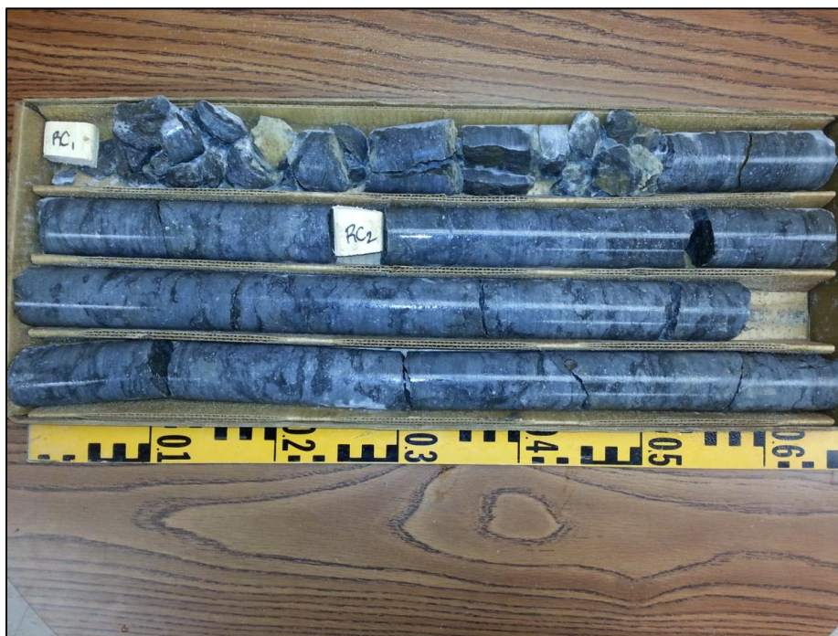
Photo 7 - Grey limestone bedrock cored between 0.6 to 2.9 m depth at BH 2.
