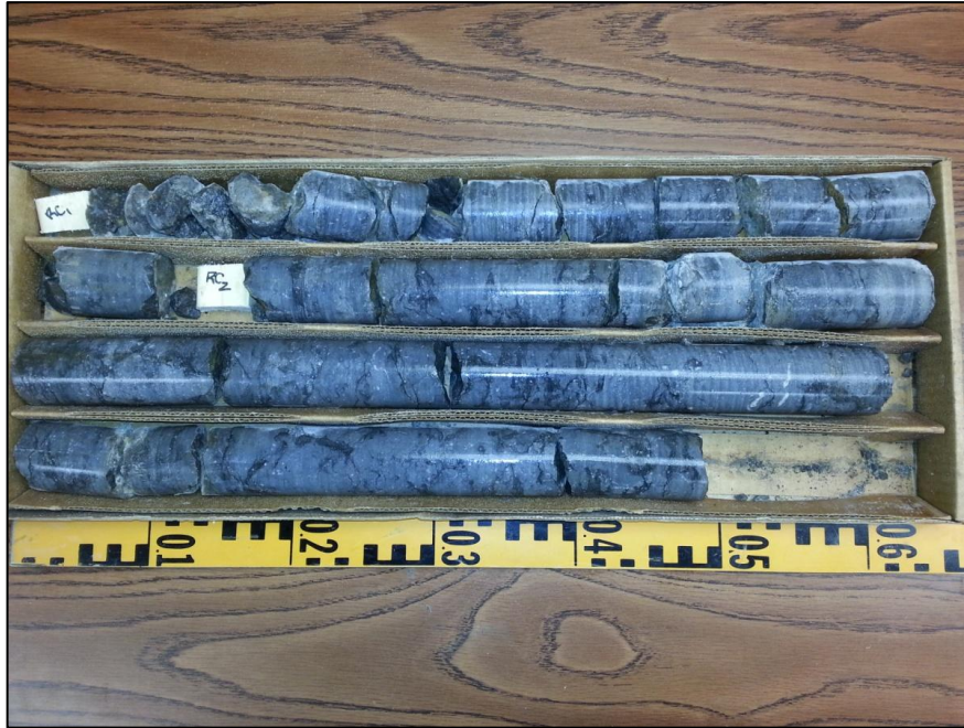
Photo 9 - Grey limestone bedrock cored between 0.9 to 3.1 m depth at BH 7.
