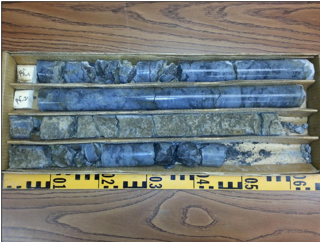
Photo 11 - Grey limestone bedrock cored between 1.1 to 3.2 m depth at BH 13.
