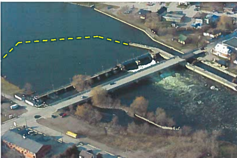
Photo 1 - Aerial Photo of Hastings Dam at Lock 18 looking downstream. Dam is to the right of Lock 18. Approximate proposed boom location is shown as yellow dashed line. Intent is to direct watercraft away from dam and towards lock. An inverted v-shape layout is proposed to promote self rescue. The boom is further set back upstream off the end of existing canal cut wall away from dam to protect against draw of main tainter gates. Currently an existing aerial cable exists upstream of dam. It is seen (lightly) in photo between dam and proposed new boom.
