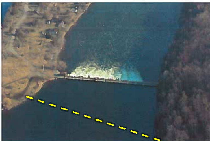
Photo 3 - Aerial Photo looking downstream. Approximate proposed boom location shown as yellow dashed line. Note that just upstream of the proposed boom at the left side is a legacy public boat launch that will remain accessible. The boom is therefore proposed to be located immediately downstream anchored at existing aerial cable anchor point. An in-water anchor will be used near the shoreline instead of approaching the private owner about using his land to install a land based anchor. With the proposed layout, the boat launch serves as a practical and safe self rescue escape point for disabled watercraft.
