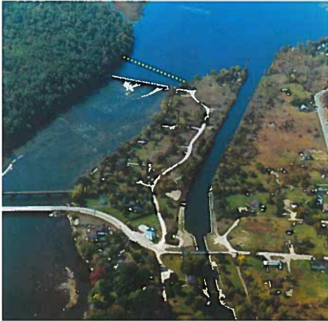
Photo 1 - Aerial Photo looking upstream. Glen Ross dam is seen at top left. Approximate proposed boom location shown as yellow dashed line. Glen Ross Lock 7 is to the right in photo. Intent of boom is to keep watercraft away from dam and directed towards lock. An angled layout is proposed to promote self rescue.
