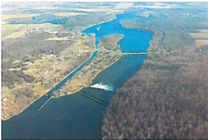
Photo 2 - Aerial Photo looking downstream. Glen Ross dam is seen at right. Approximate proposed boom location shown as yellow dashed line. Glen Ross Lock 7 seen to the left is accessed via a canal cut. Intent of boom is to keep watercraft away from dam and directed towards lock.
