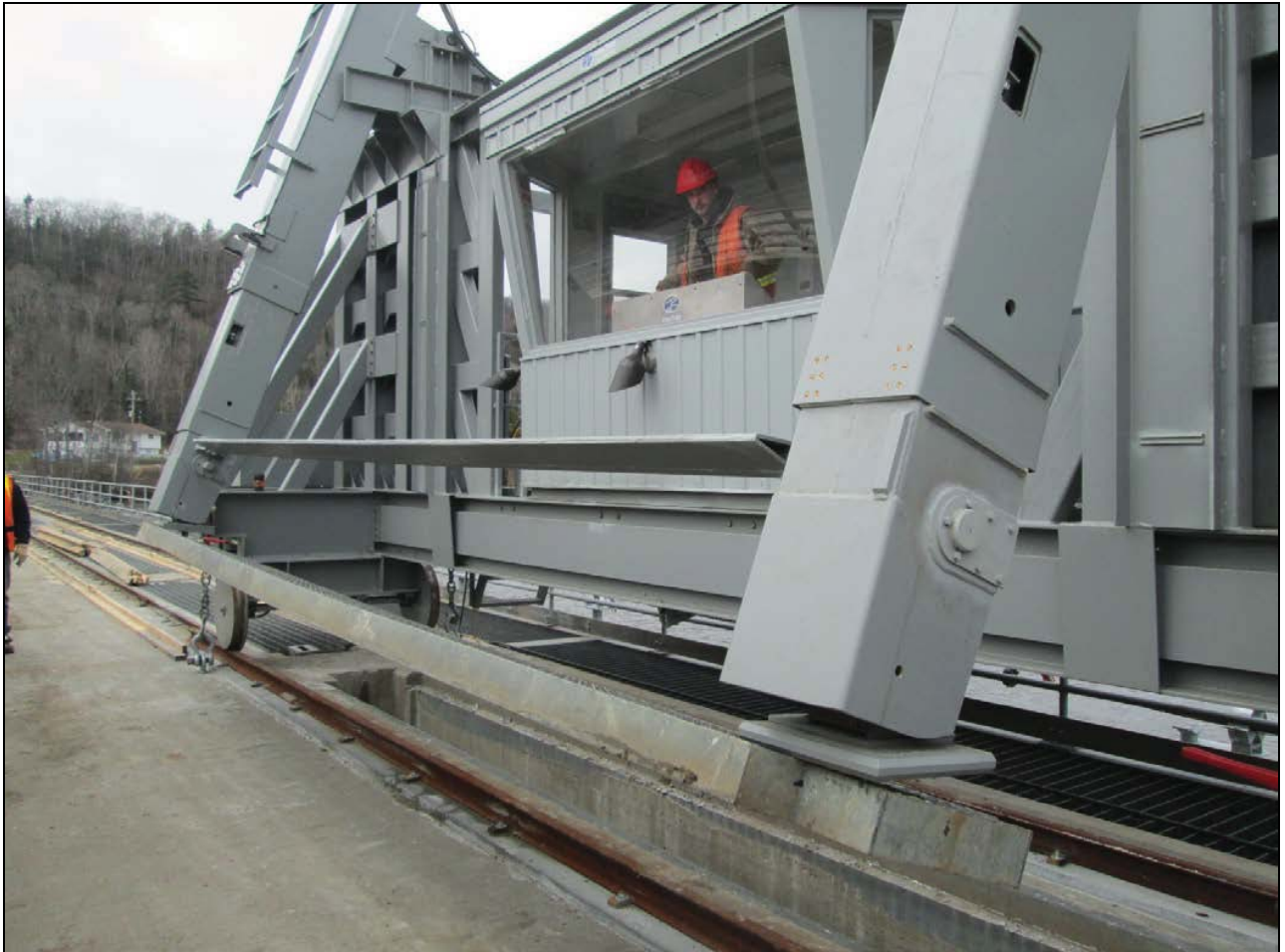
Figure 1 - Stoplog lifter, downstream side, with booms in the process of lifting out a sluice grate. Note lack of any overhang above the window.
