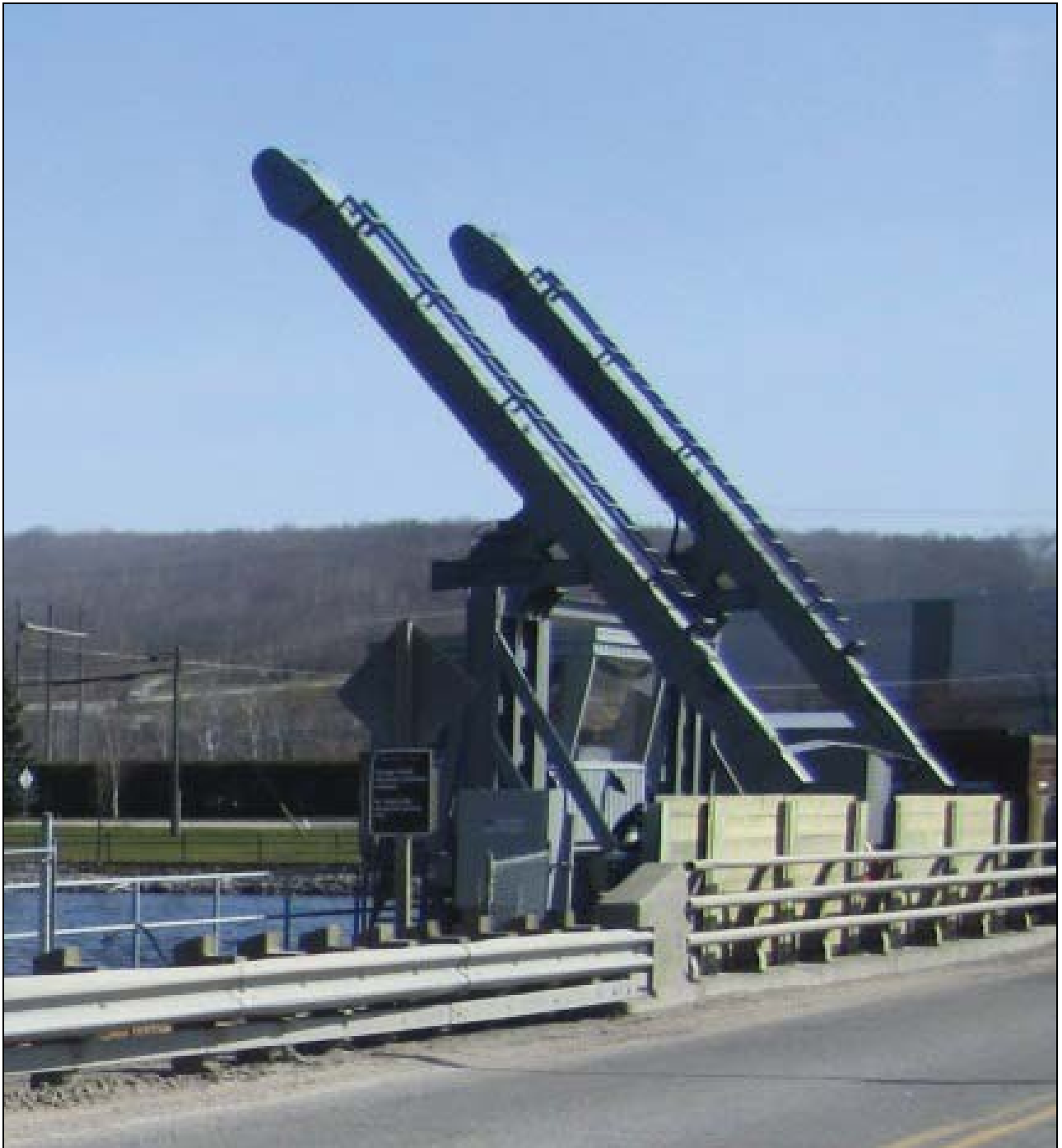
Figure 6 - Ontario dam's stoplog lifter showing angle of booms when picking up stoplog from the stack on the operations deck.
