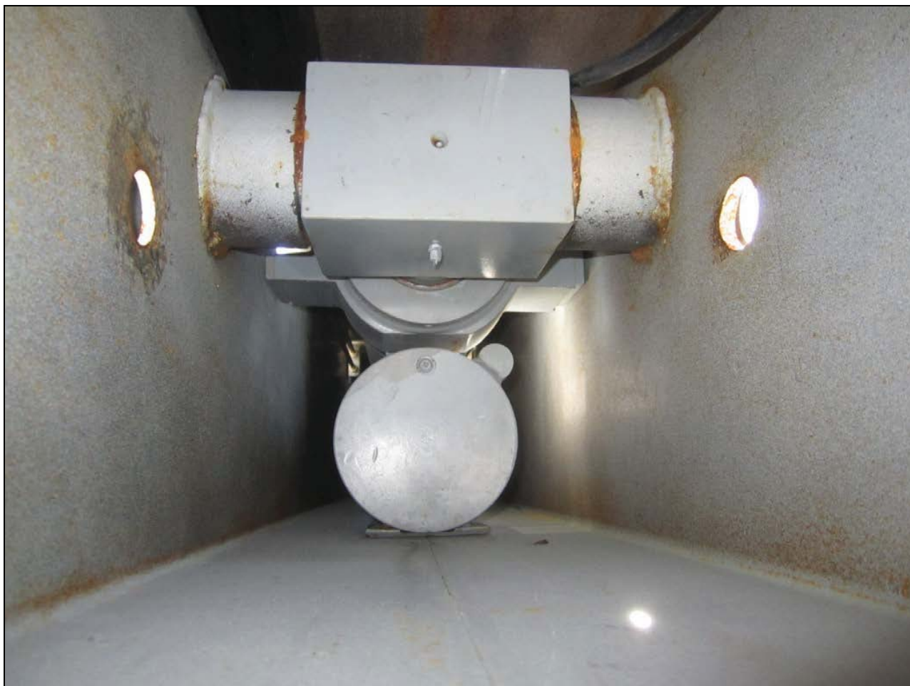
Figure 8 - Stoplog lifter, looking up inside boom from just above the harpoon hooks.
