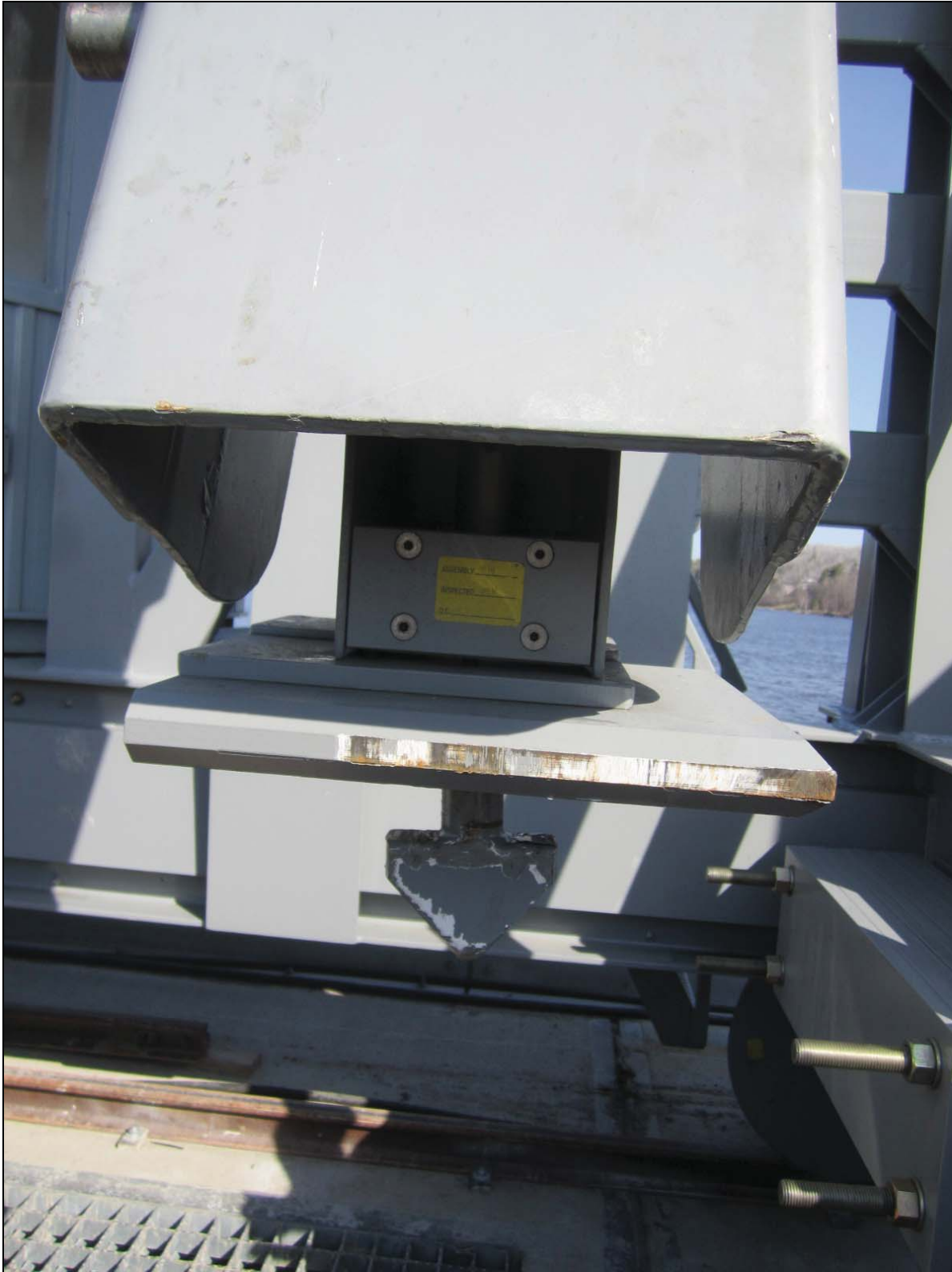
Figure 7 – Stoplog lifter, typical detail of boom end showing harpoon hook.
