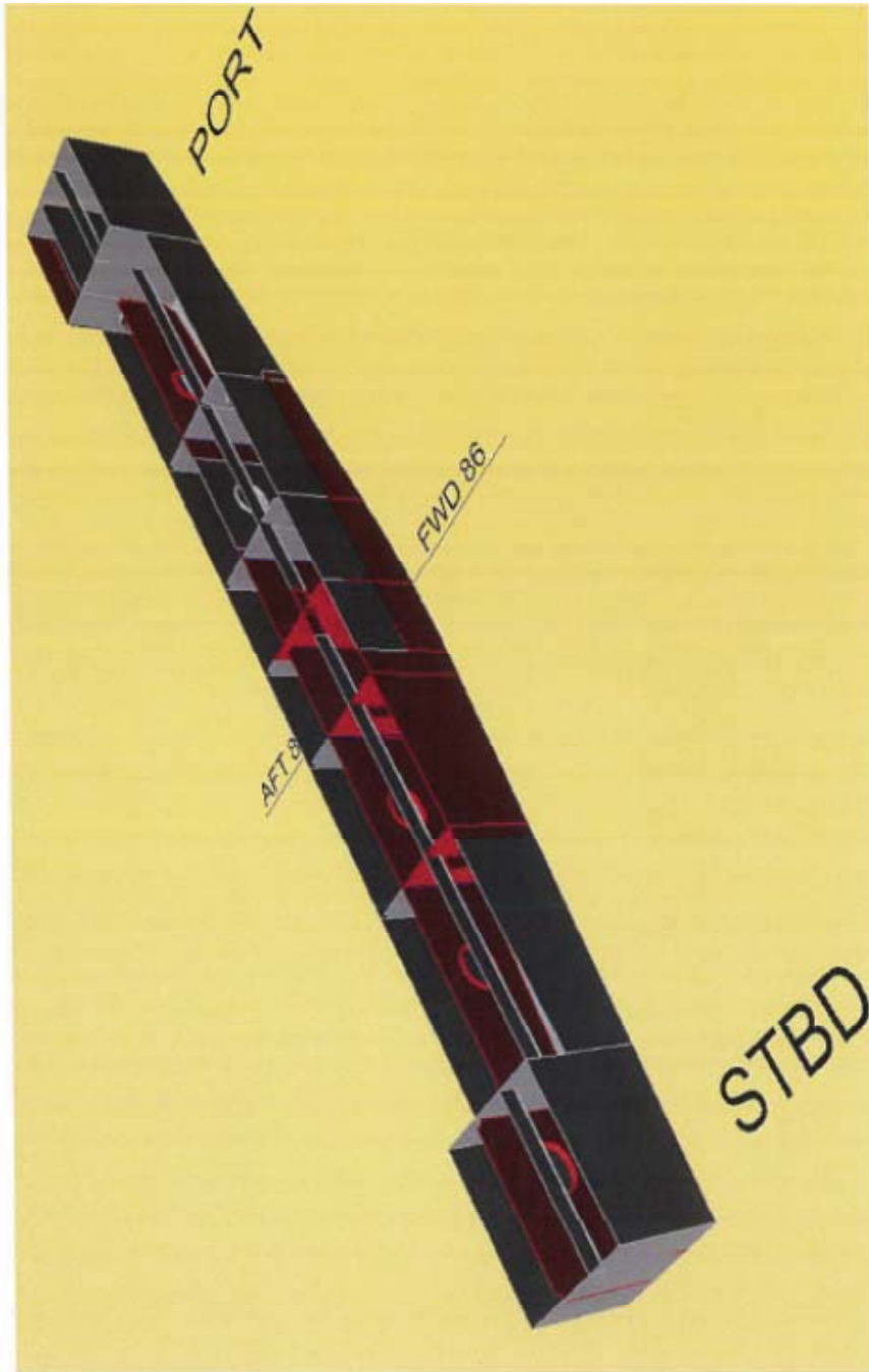
View Looking Aft (tanktop plating not shown for clarity)
