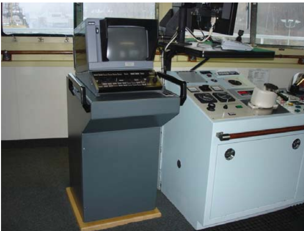
Picture 4: S Band Radar Location for cable run
