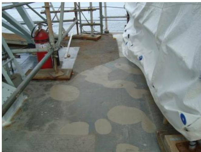
Missing Non-skid on Bridge Top
