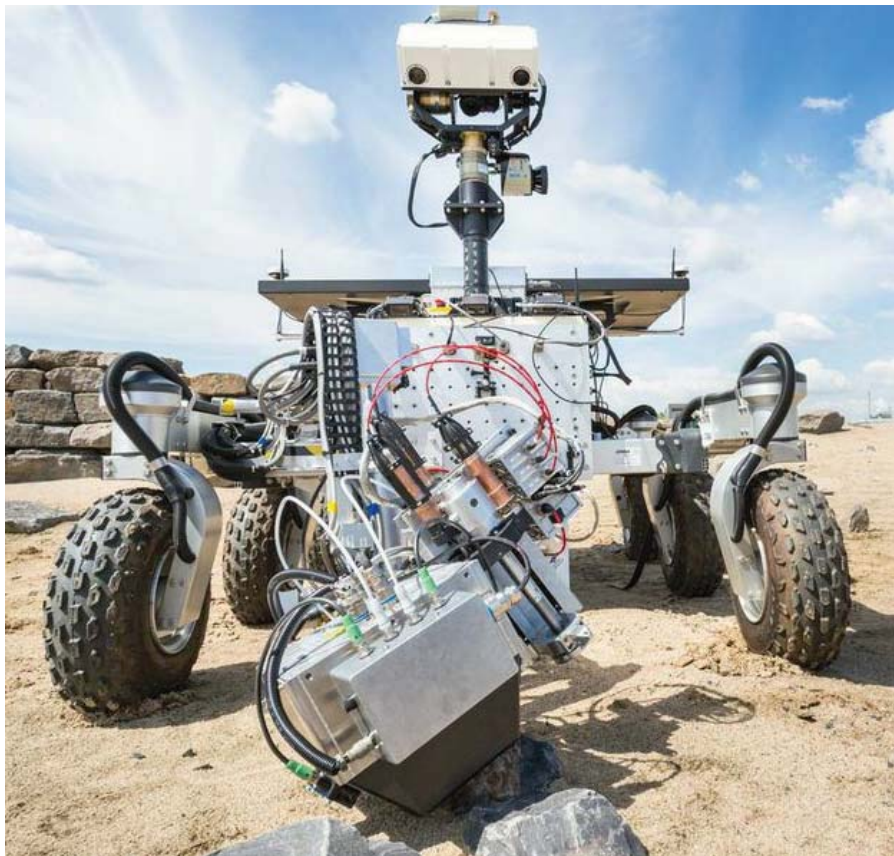
Figure 1: Mini-Corer at the end of the Small Manipulator on the Mars Exploration Rover prototype
