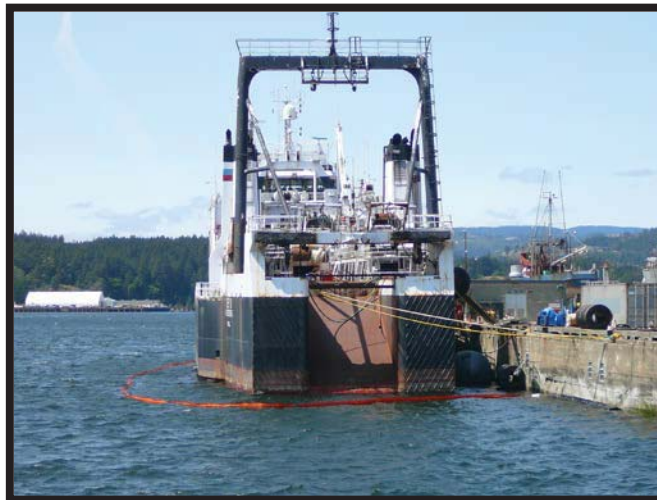
Containment boom around vessel during fueling operations
