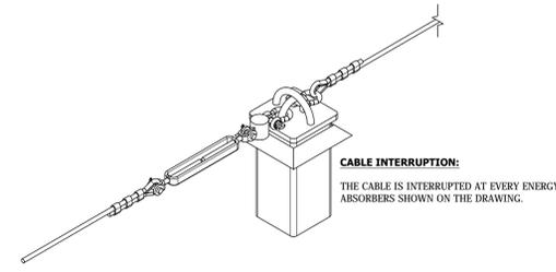
DETAIL 05 - ASSEMBLY - HORIZONTAL CABLE W/ ENERGY ABSORBER
