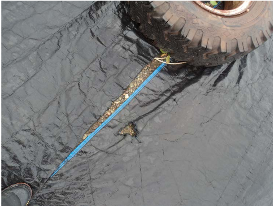
Photo 3. Tear along seam of covering tarp.
