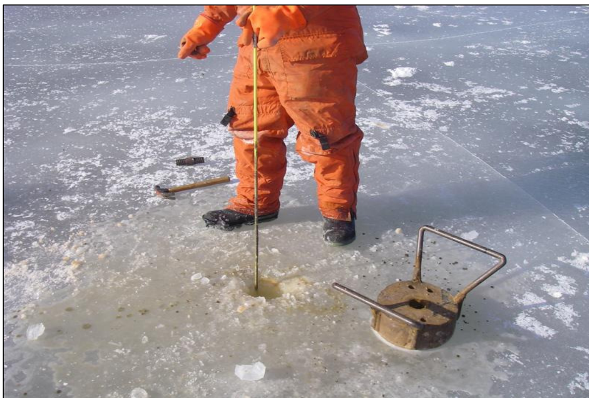
Photo 2 - Probing Pond Bottom Sediments - Feb. 6, 2007 PRSS-07BH-01 (Coordinates: 5124120, 4599200)
