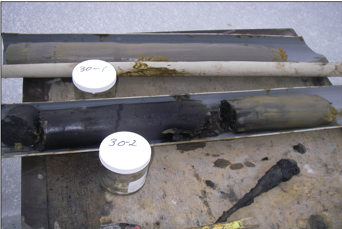
Photo 10 - Interface between Grey Silt and Clay and Black Coal Fines Layers PRSS-07BH-30-01 and PRSS-07BH-30-02 (Coordinates: 5124163, 4599184) (Coordinates: 5124196, 4599175)
