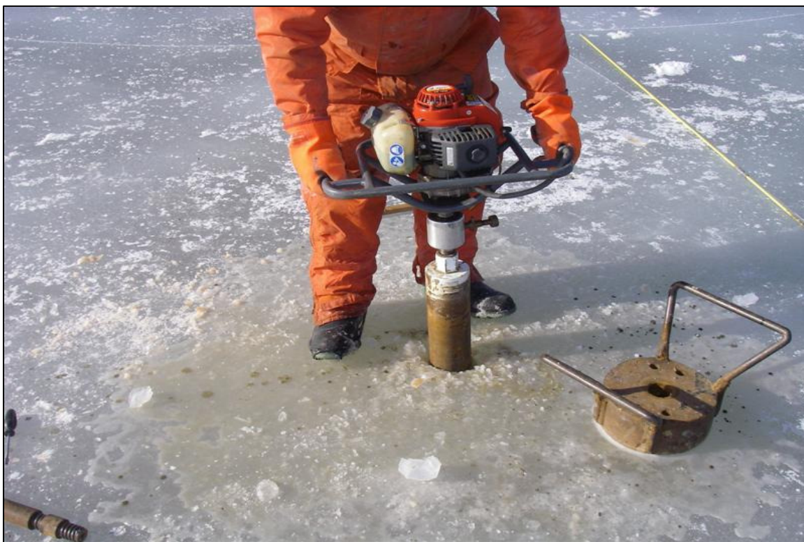
Photo 1 - Coring Ice to Access Pond Bottom - Feb. 6, 2007 PRSS-07BH-01 (Coordinates: 5124120, 4599200)
