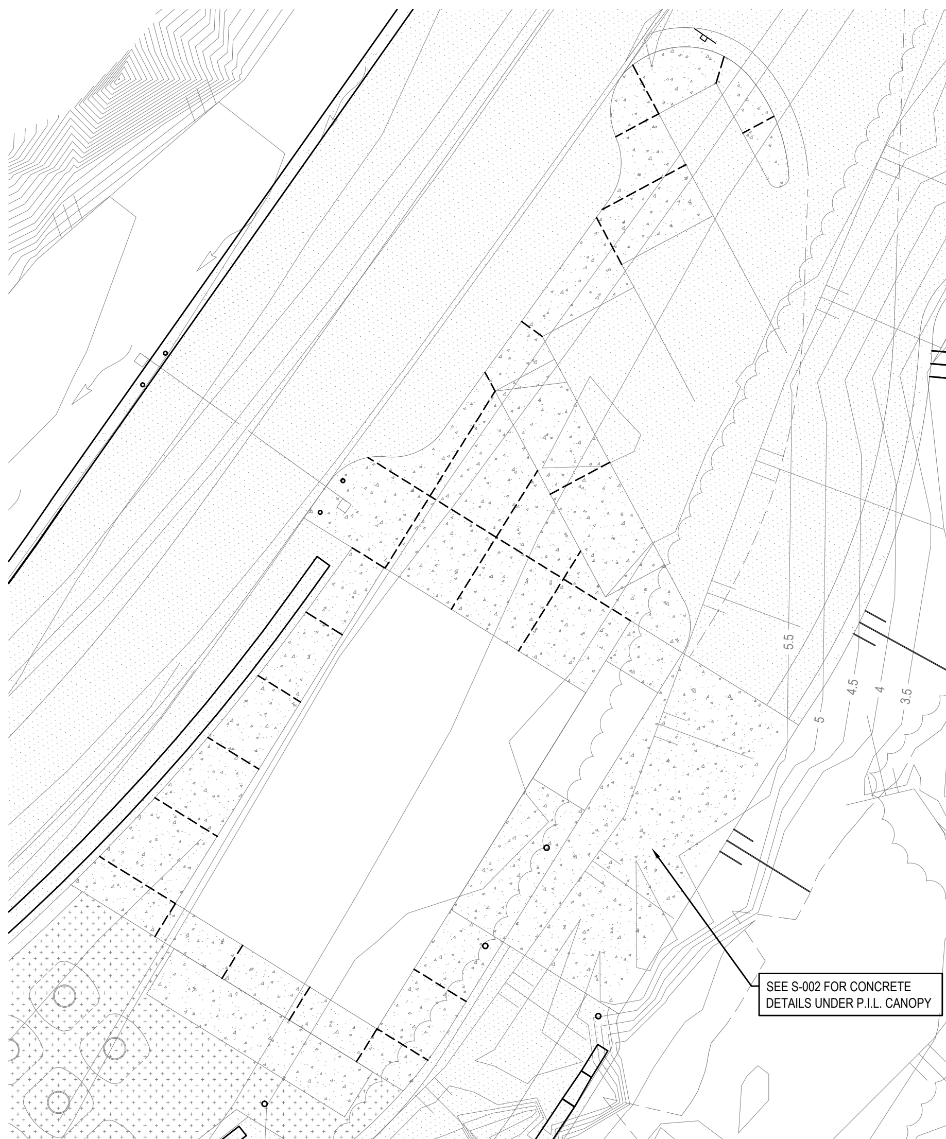
CONCRETE CONSTRUCTION CONTROL JOINTS SCALE: 1:150
