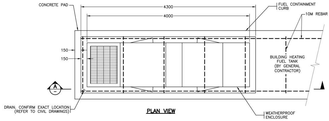
NOTE: CONFIRM EXACT DIMENSIONS WITH GENERATOR MANUFACTURER AND BUILDING HEATING FUEL TANK SUPPLIER PRIOR TO CONCRETE PAD FABRICATION.
