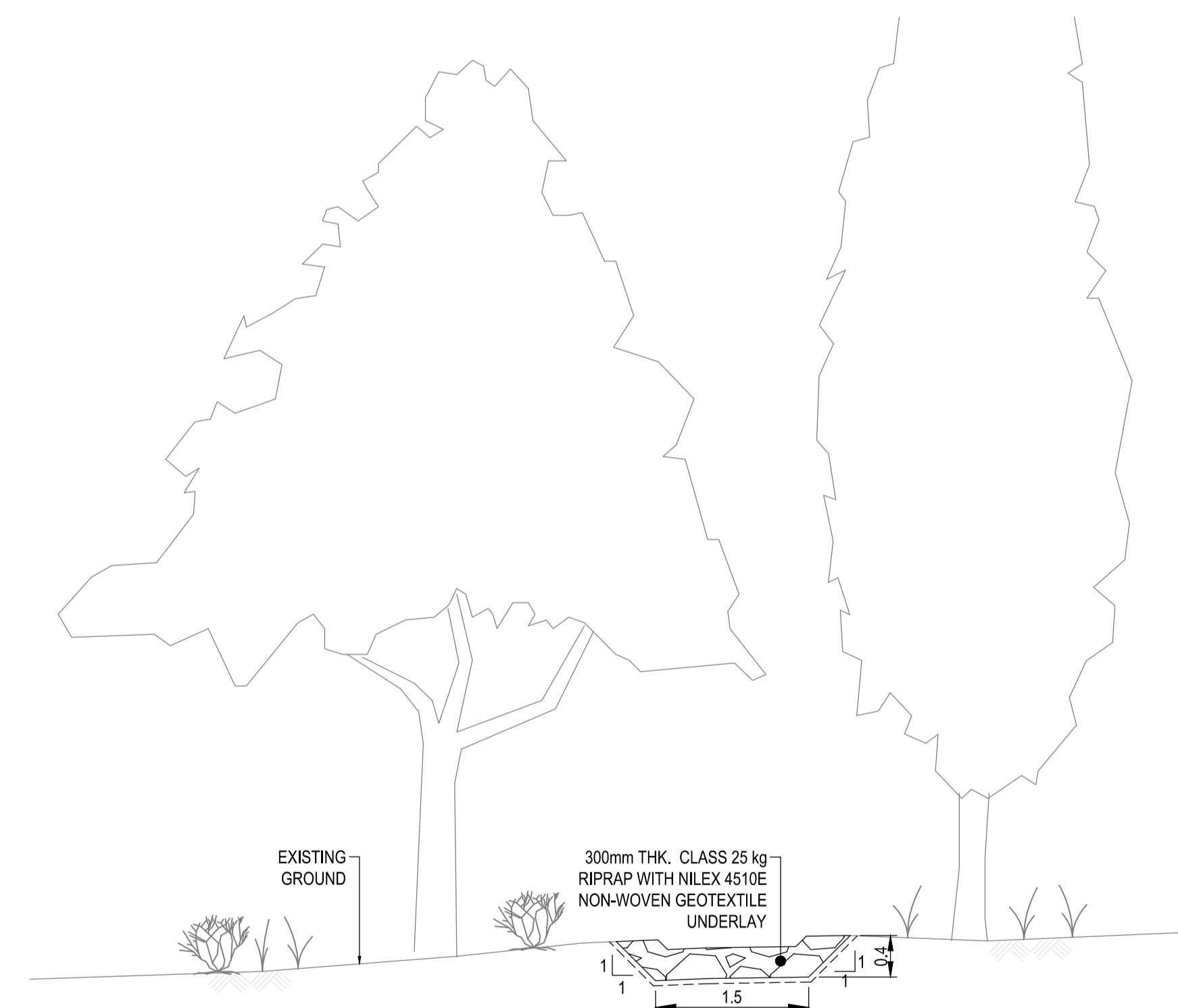
SECTION 3 TYPICAL SECTION PROPOSED CLASS 25 kg RIPRAP DRAINAGE SLOPE SCALE: 1:50
