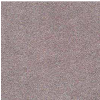
C HB2½ Rust grade C Hydroblasted to an Sa2½ equivalent
