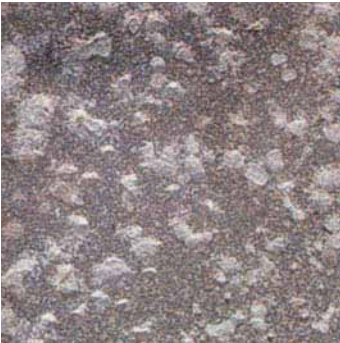
D HB2½ Rust grade D Hydroblasted to an Sa2½ equivalent
