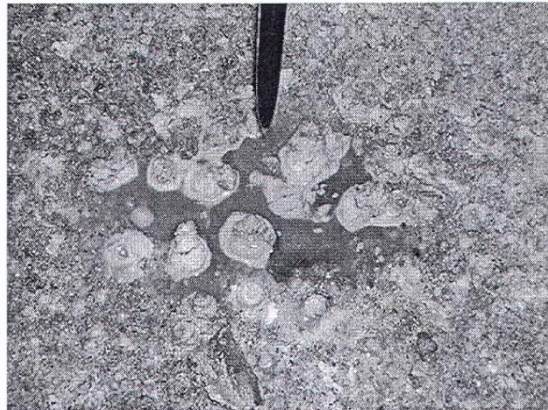
Figure 14 - Copper Ions Deposited on Aluminum Causing Corrosion
