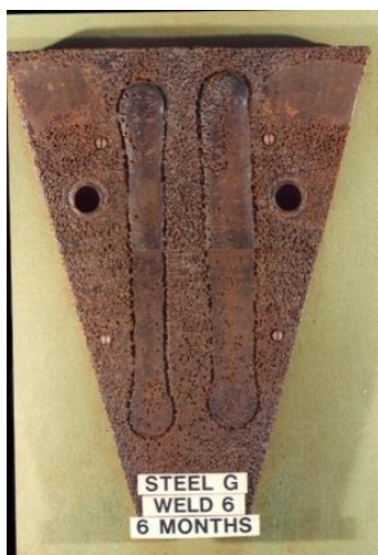
Figure 16 - HAZ Corrosion
