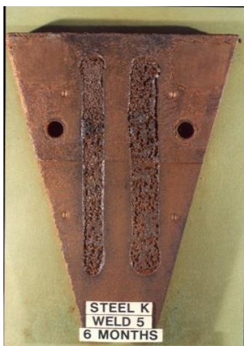
Figure 15 - Weld Metal Corrosion
