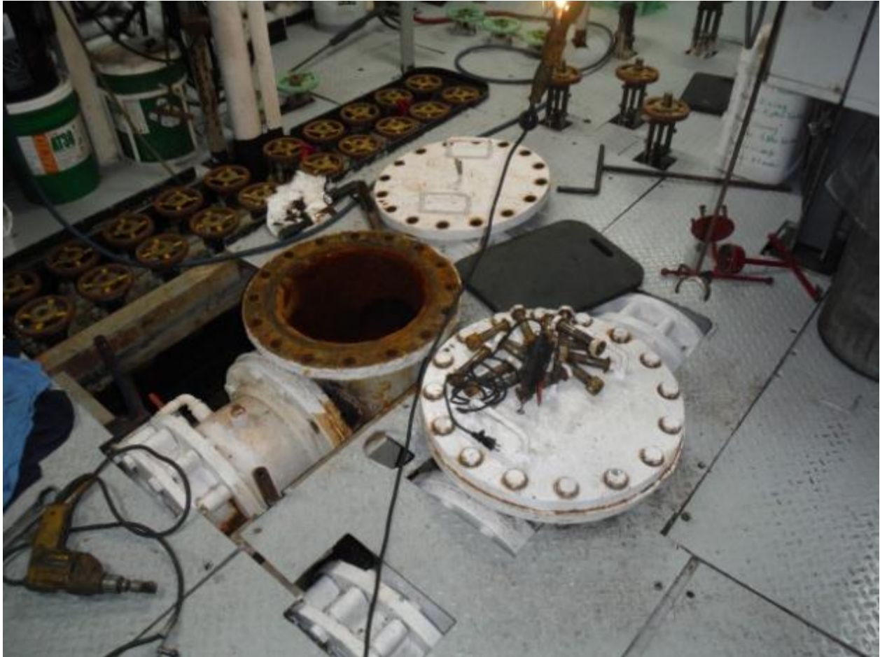
Figure 1 - Both Strainers, forward strainer with cover removed.
