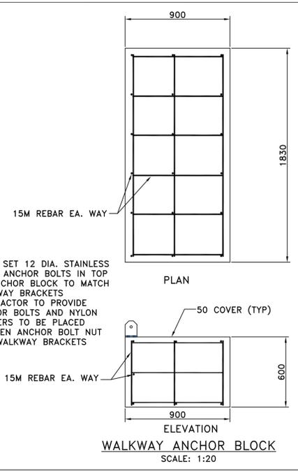
NOTE: SET 12 DIA. STAINLESS STEEL ANCHOR BOLTS IN TOP OF ANCHOR BLOCK TO MATCH WALKWAY BRACKETS. CONTRACTOR TO PROVIDE ANCHOR BOLTS AND NYLON WASHERS TO BE PLACED BETWEEN ANCHOR BOLT NUT AND WALKWAY BRACKETS
