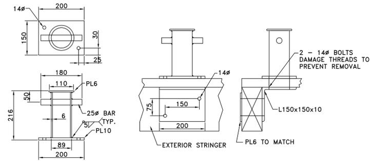
BOLLARD AND BOLLARD MOUNTING DETAILS - 6 REQ'D
