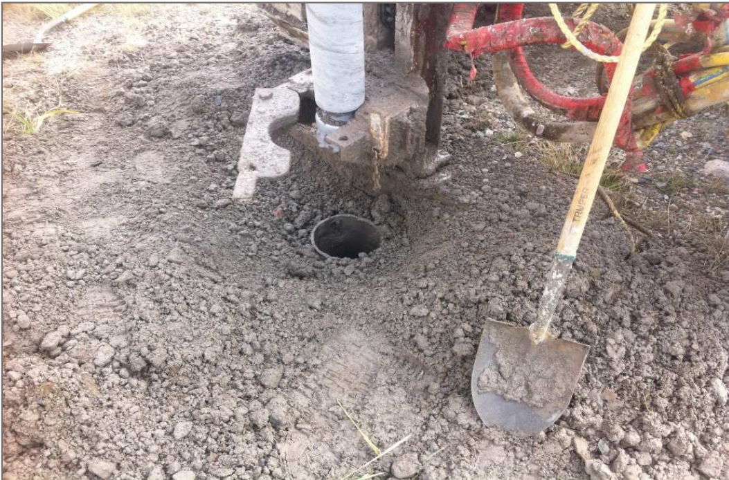
Photo 8: The disturbed soil cuttings blown from Probehole 2 can be seen around the cased probehole.
