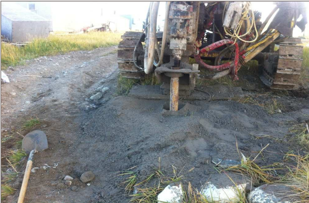
Photo 10: The disturbed soil cuttings blown from Probehole 3 can be seen around the cased probehole.
