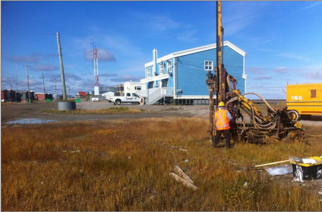
Photo 7: Facing northeast through the project as the driller begins drilling Probehole 1 within the marshy area of the site.
