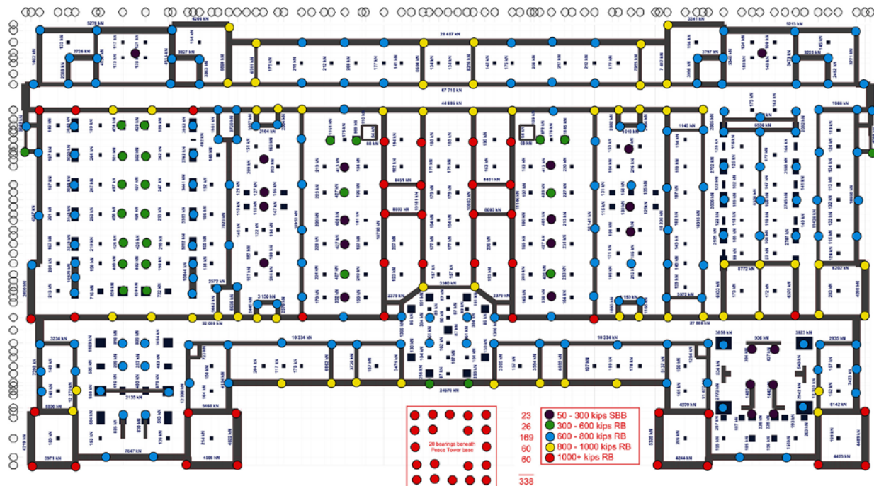
Figure 9 - Base isolator potential layout plan
