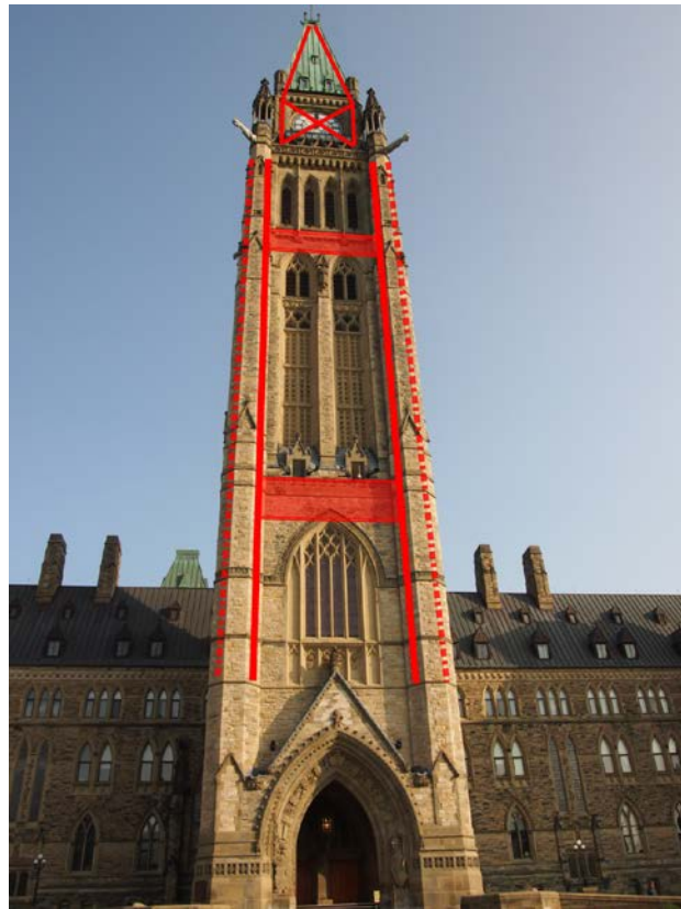
Figure 7 - Schematic layout of Peace Tower reinforcing
