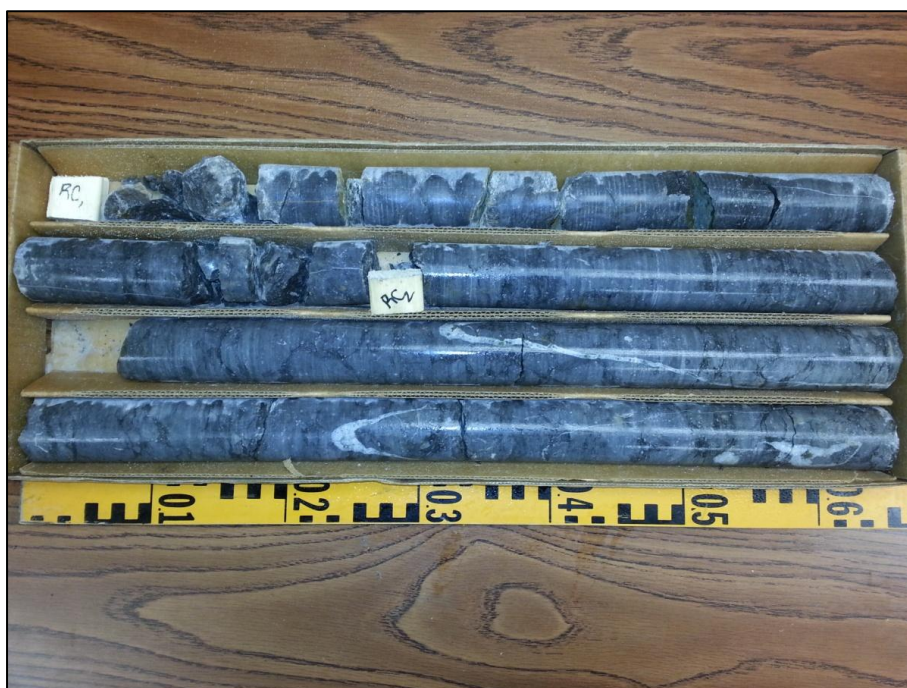
Photo 8 - Grey limestone bedrock cored between 0.8 to 3.1 m depth at BH 5.
