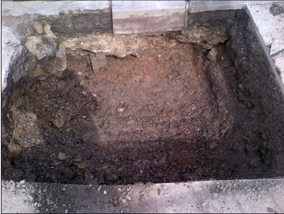
Photo 3 - Soil profile along north side of test pit and existing wall foundation exposed at TP 7A.
