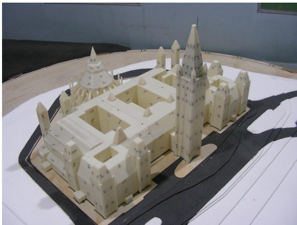
PHOTOGRAPH 4: DETAILED VIEW OF PRESSURE INTEGRATION MODEL
