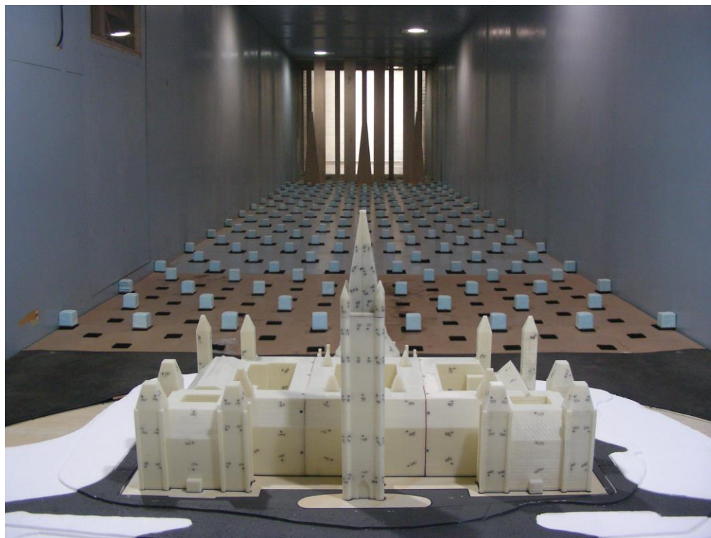
PHOTOGRAPH 3: 1:250 SCALE MODEL IN GWE WIND TUNNEL, LOOKING UPWIND
