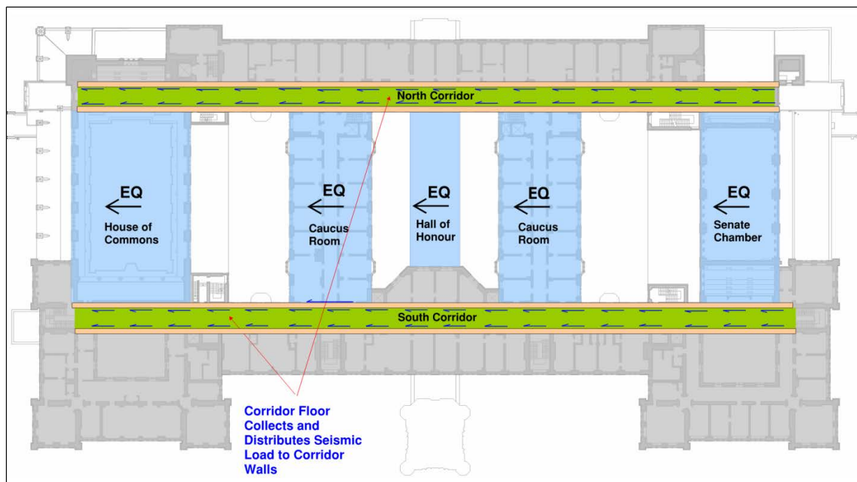
Figure 6.11: Corridor Diaphragm Collectors
