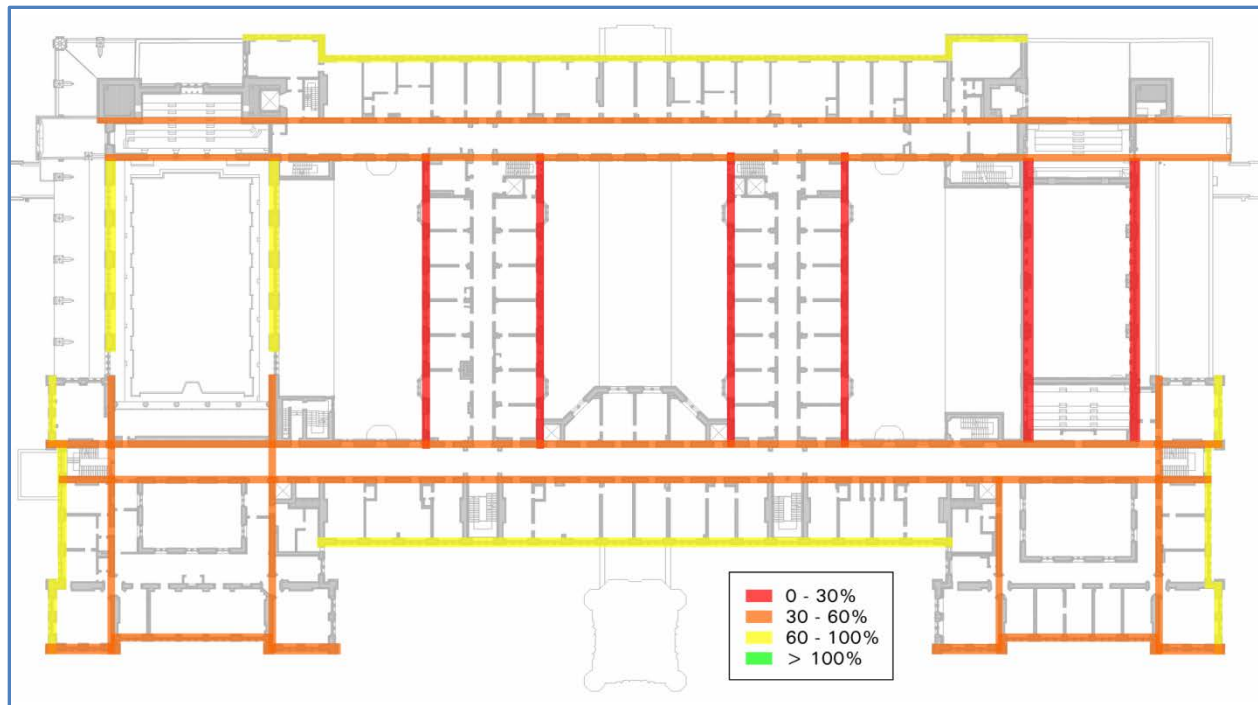
Figure 6.4: L3 to Roof (Combined) – Wall Capacity/Demand Ratios (2010 NBCC)
