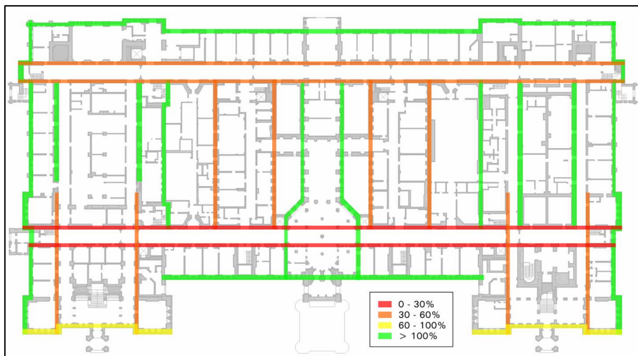
Figure 6.5: L1 and L2 (Combined) – Wall Capacity/Demand Ratios (2010 NBCC)
