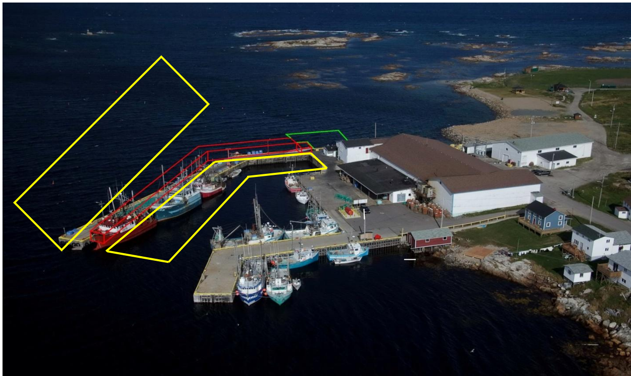
Figure 3: Aerial close-up of wharf to be reconstructed (in red) and infill area (green). Approximate dredge areas in yellow.
