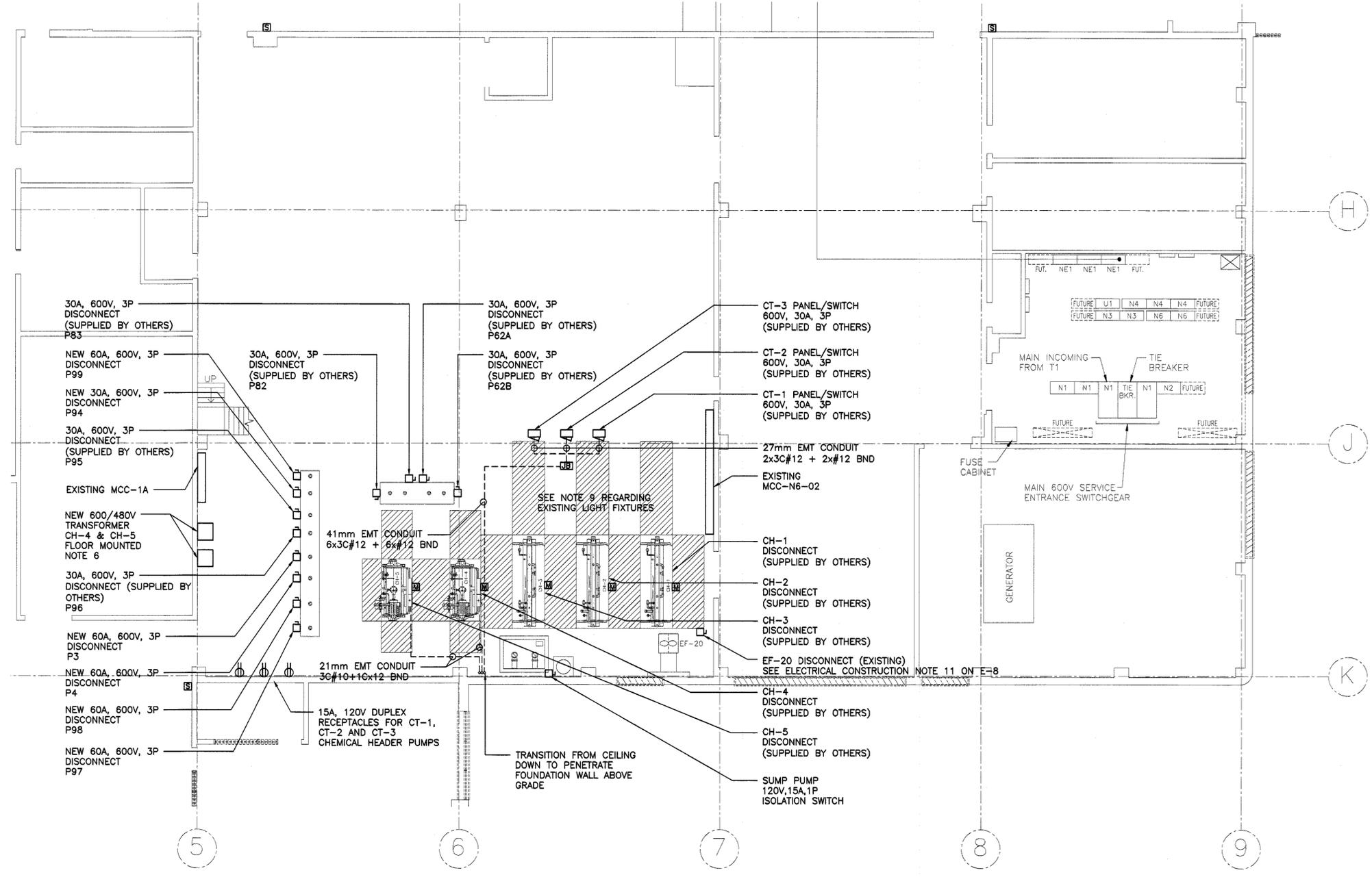
**PLAN - ELECTRICAL EQUIPMENT (NEW CONSTRUCTION)**
