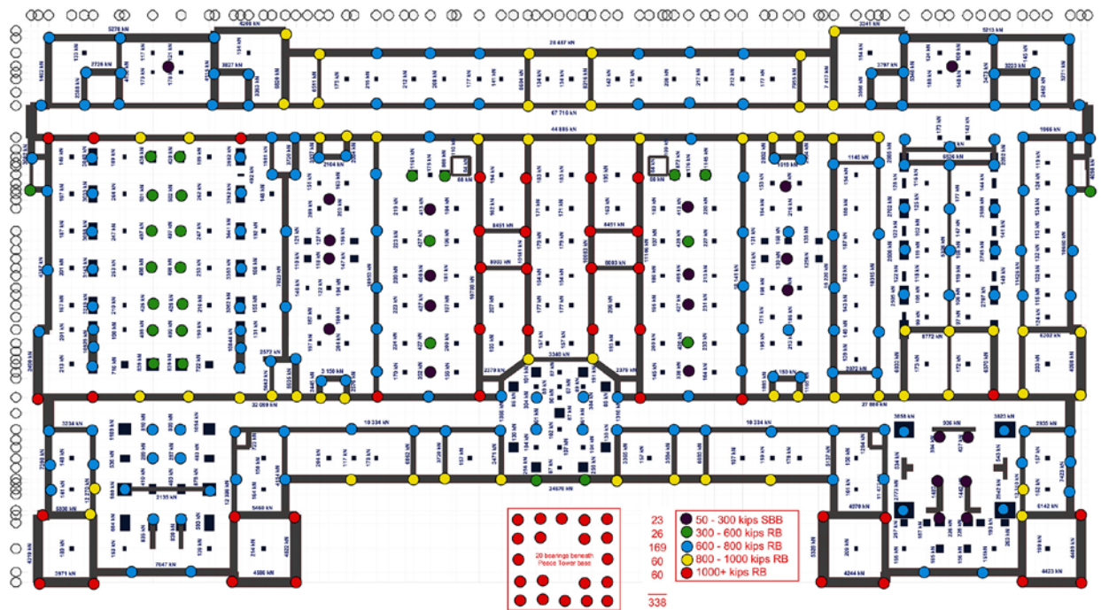
Figure 9 - Base isolator potential layout plan
