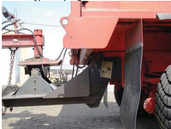
Fifth Wheel-Type Coupling
