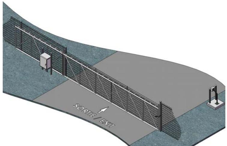
maximum opening/closing movement time is reached. The gate can be activated by push-buttons, remote control, keypad, card reader or any other similar device. Also, all security devices such as safety edges, loops and photoelectric cell can be connected to the control panel.
