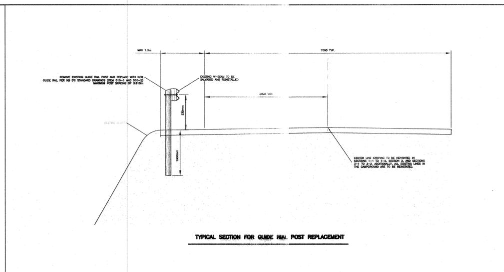
TYPICAL SECTION FOR GUIDE RAIL POST REPLACEMENT
