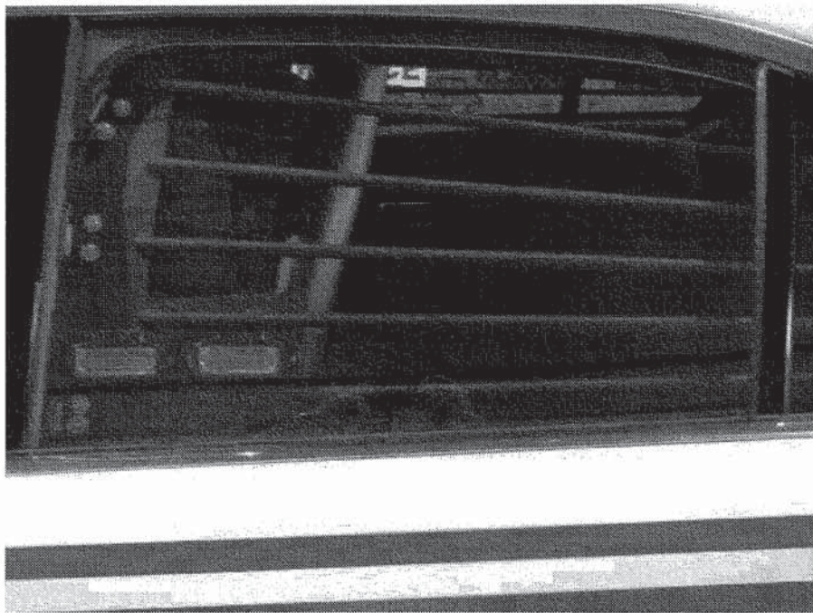
Figure 26 – Window barriers with window-mounted intersection lights
