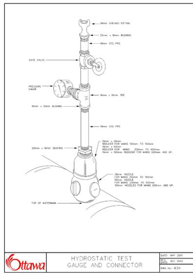
**Hydrostatic Test Gauge and Connector**
