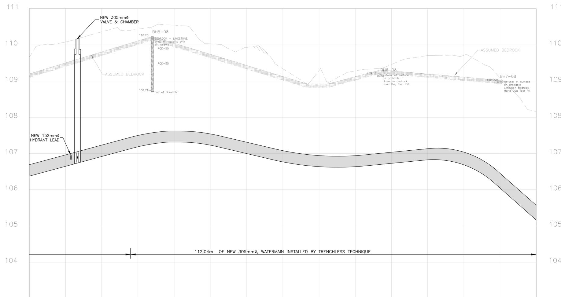
NOTE: FOR TRENCHLESS INSTALLATIONS, VERTICAL AND HORIZONTAL BENDS MAY BE REPLACED WITH PIPE DEFLECTIONS PROVIDED RESULTANT PIPE DEFLECTIONS DO NOT EXCEED MANUFACTURERS' RECOMMENDATIONS.
