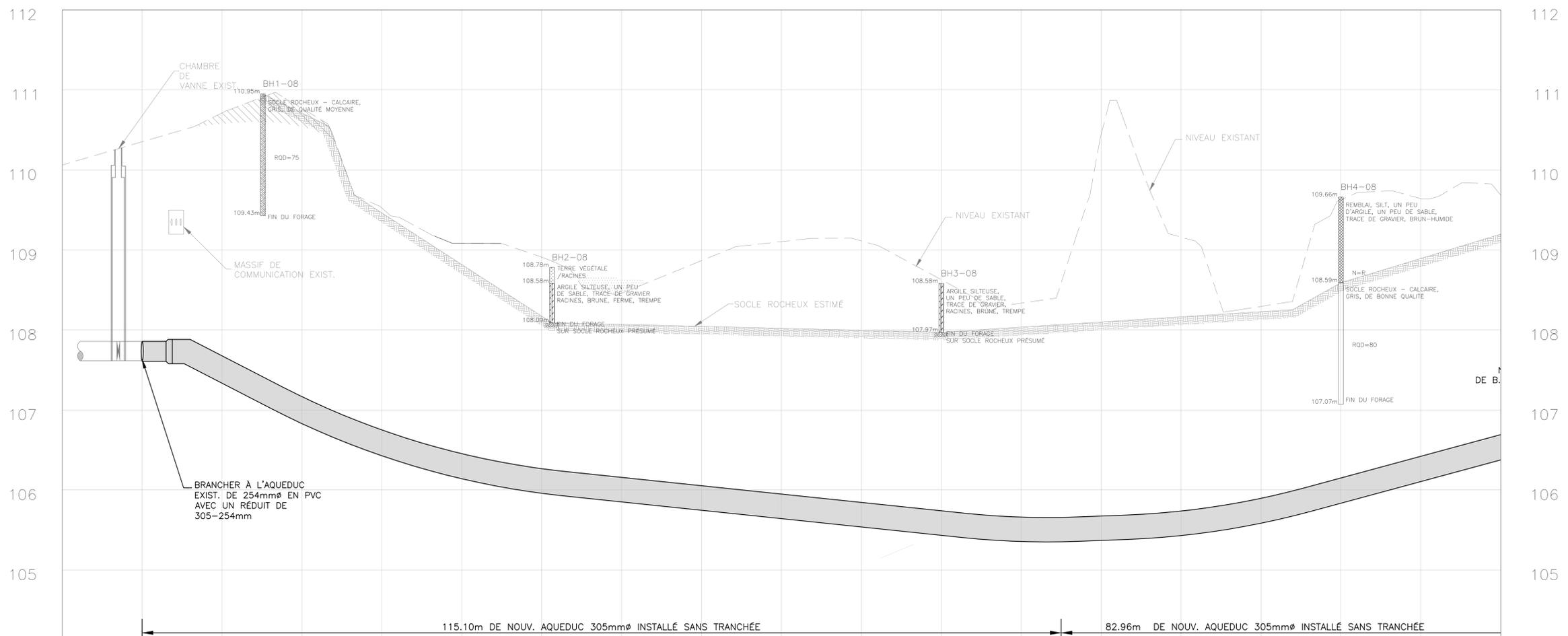
NOTE: POUR L'INSTALLATION SANS TRANCHÉE, LES COUDES VERTICAUX ET HORIZONTAUX PEUVENT ÊTRE REMPLACÉS PAR DES DÉFLECTIONS DE LA CONDUITE QUI N'EXCÈDENT PAS LES RECOMMANDATIONS DU MANUFACTURIER.
