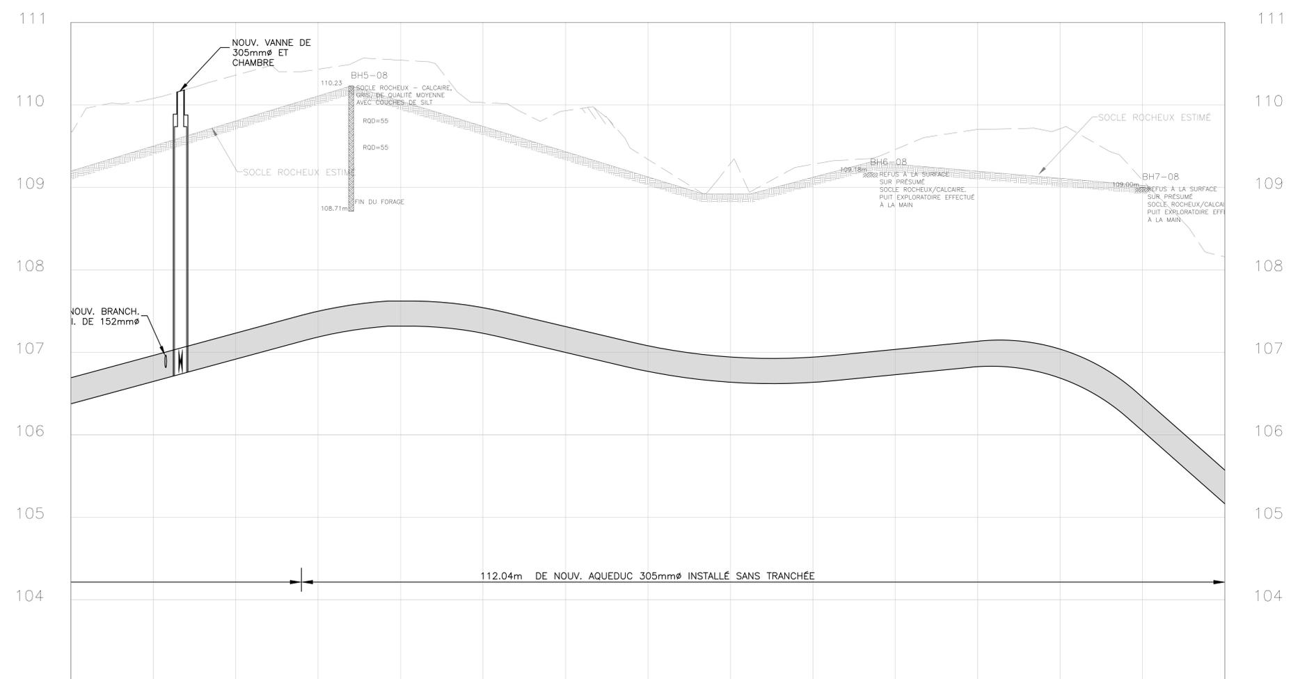
NOTE: POUR L'INSTALLATION SANS TRANCHÉE, LES COUDES VERTICAUX ET HORIZONTAUX PEUVENT ÊTRE REMPLACÉS PAR DES DÉFLECTIONS DE LA CONDUITE QUI N'EXCÉDENT PAS LES RECOMMANDATIONS DU MANUFACTURIER.
