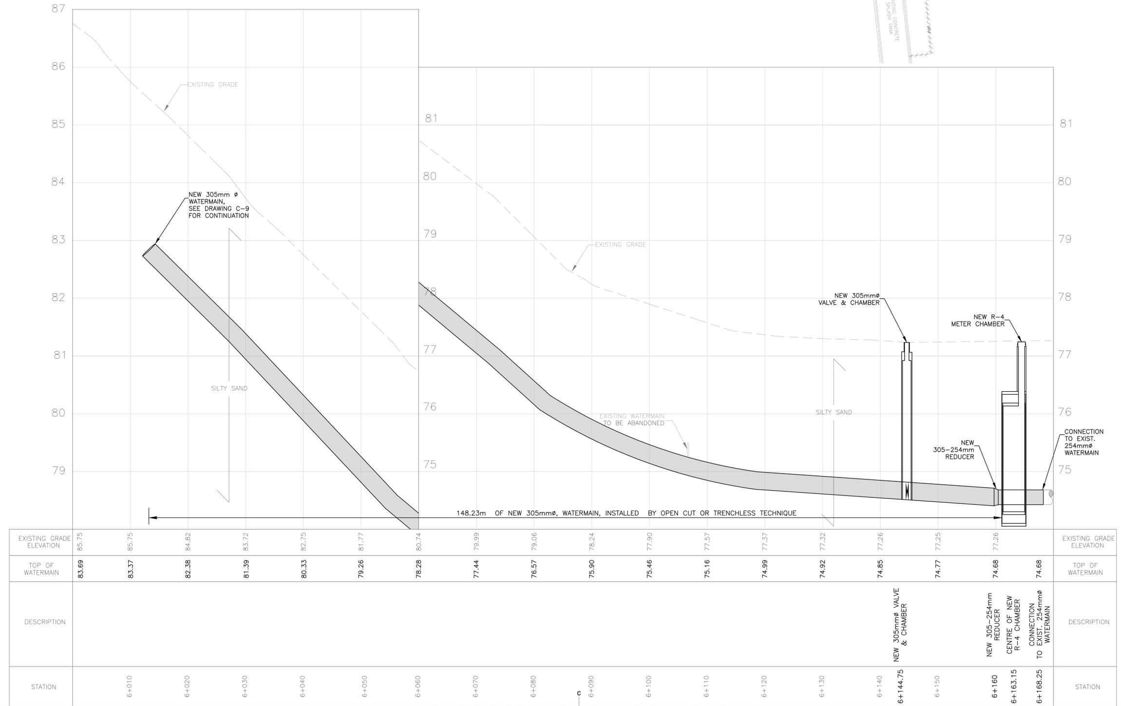
NOTE: FOR TRENCHLESS INSTALLATIONS, VERTICAL AND HORIZONTAL BENDS MAY BE REPLACED WITH PIPE DEFLECTIONS PROVIDED RESULTANT PIPE DEFLECTIONS DO NOT EXCEED MANUFACTURERS' RECOMMENDATIONS.
