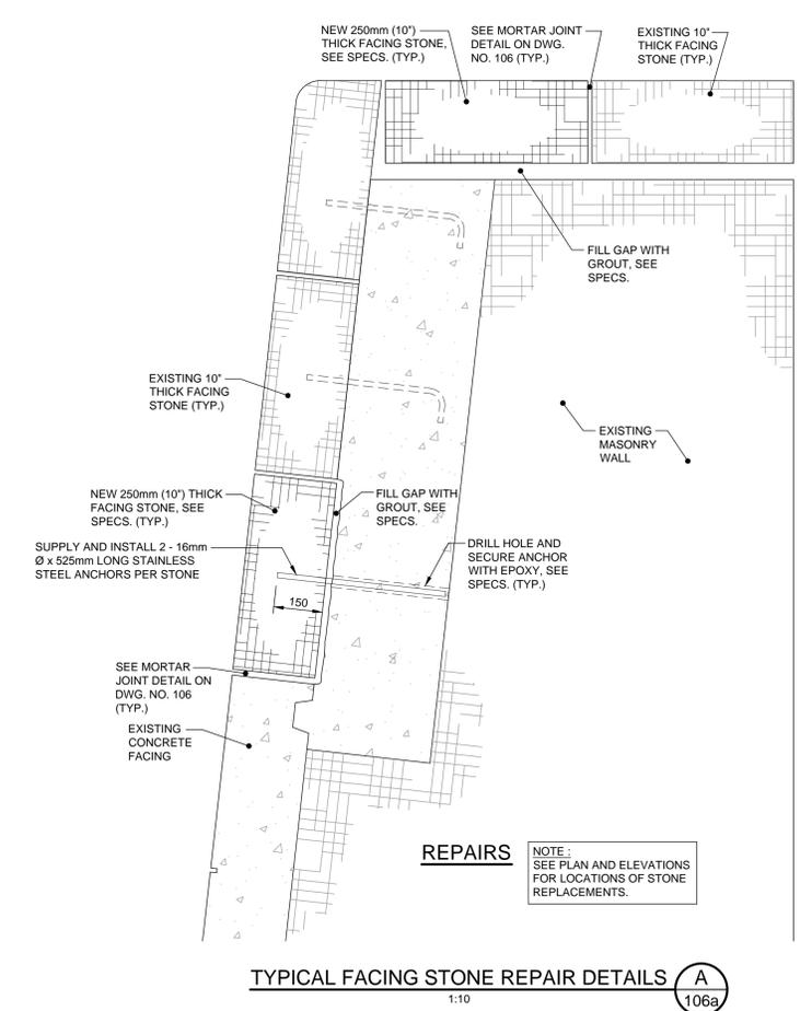
**TYPICAL FACING STONE REPAIR DETAILS** A 106a
