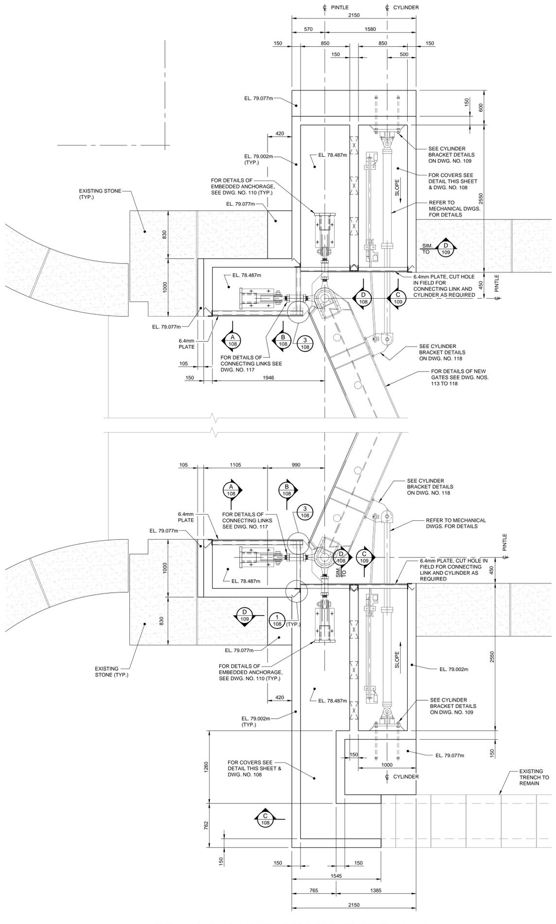
**TOP ANCHORAGE AND CYLINDER PIT REINSTATEMENT PLAN**
