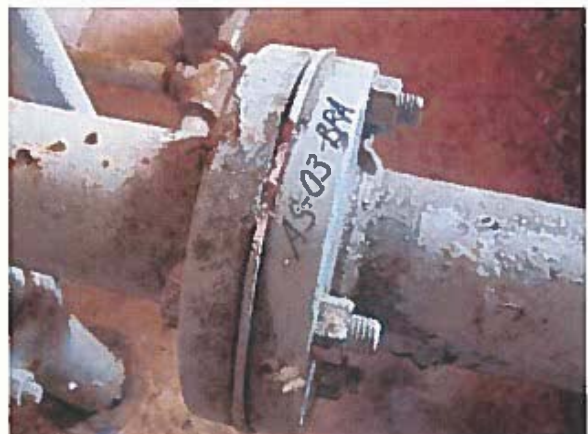
Photo 4: Photo of sample AS-03-BRA, gasket material on a pipe flange.
