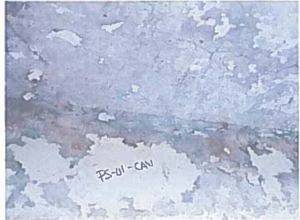
Photo 8 – Photo of paint sample P-01-CAV, white exterior trim paint (lead 3640 mg/kg, mercury 25.3 mg/kg). PS-01-CAV was determined to be lead leachate hazardous.
