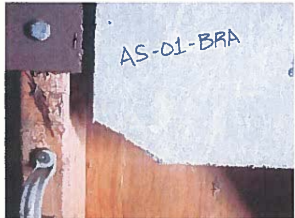
Photo 2: Photo of sample AS-01-BRA, two sections of wall board (containing 15% chrysotile).
