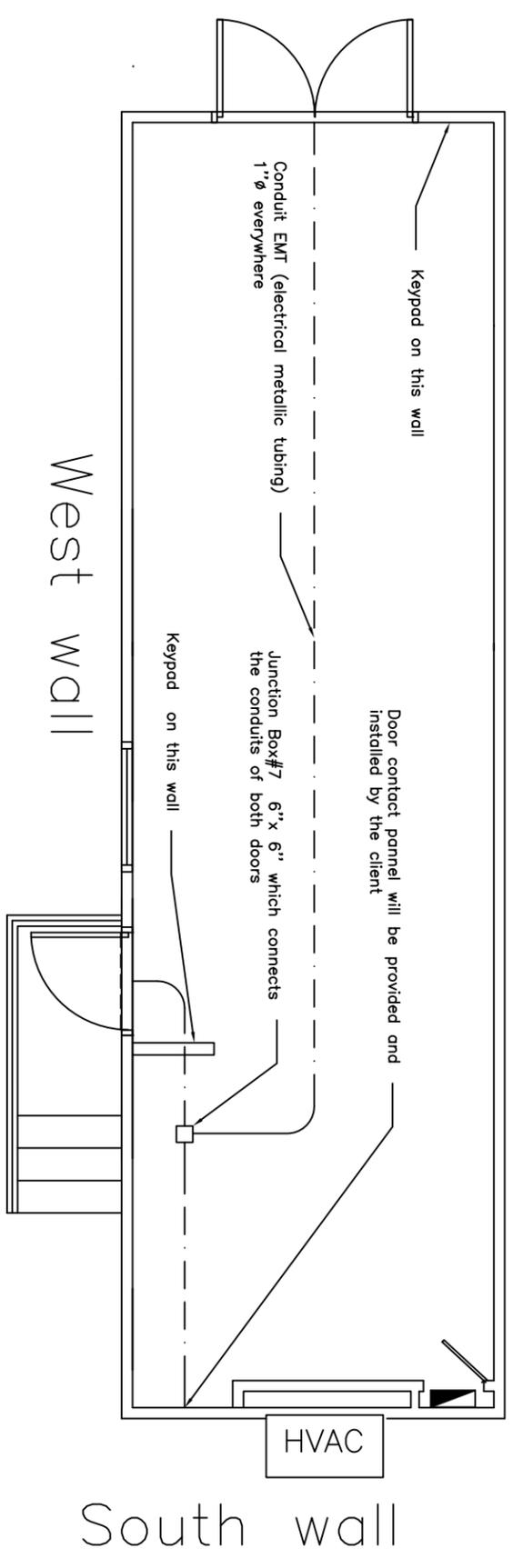
Détails of the conduits and junction boxes for the doors' contact
